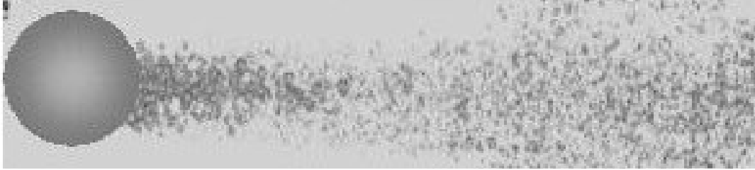
Figure 2: Droplet breakup process in an accelerating flow field; We > 12
