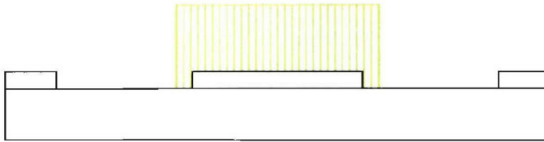
Fig. 4: Patterning PI-2737 to form MESA bridge.
