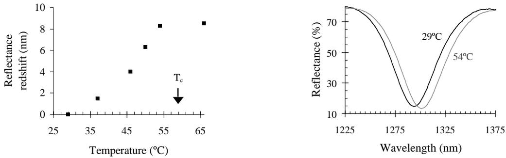
**Figure 3.** (a) Reflectance redshift of tunable porous silicon one-dimensional photonic bandgap microcavity resonance as a function of temperature. The shift saturates at the phase transition temperature ( $T_c$ ) of the infiltrated liquid crystals. (b) Reflectance spectra of microcavity resonance at two different temperatures.
