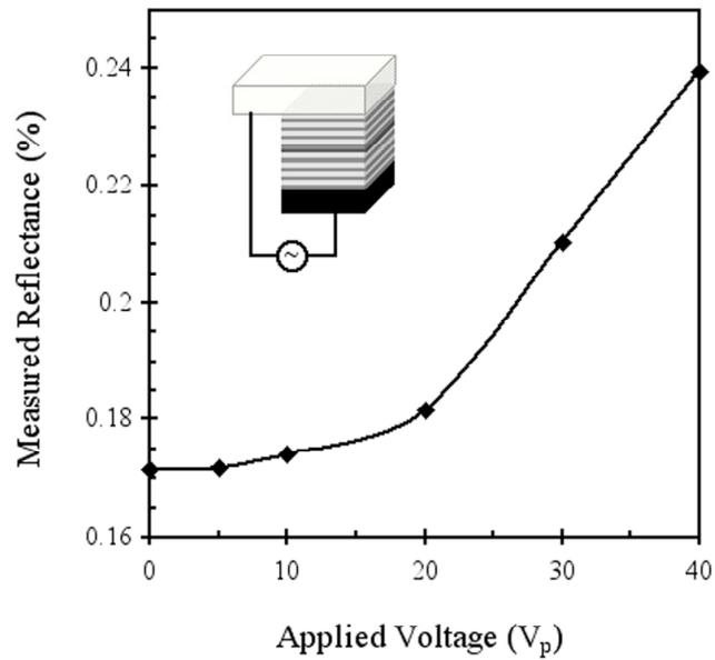
**Figure 8:** First demonstration to true electrical tuning in a 1-D PBG microcavity structure. Note the large voltage required, which results from (1) the use of small pores which makes liquid crystal rotation difficult, and (2) the presence of a liquid crystal layer between the top electrode and the PBG itself.
