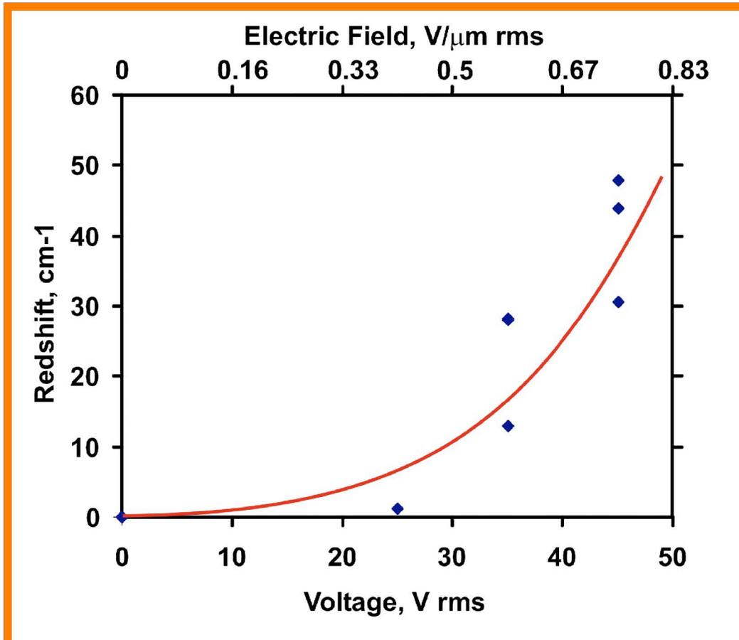
**Figure 9:** Switching of a 2-D PBG structure filled with liquid crystal molecules has been achieved for modest electric fields. Once the structures are fabricated in SOI, the layer thickness is expected not to exceed  $1 \mu\text{m}$  and the switching voltage should be 1 V or less. Note that this result was achieved with a 2-D PBG membrane that did not have a resonant defect structure. On going effort is focusing at repeating this result with 2-D PBG microresonators.
