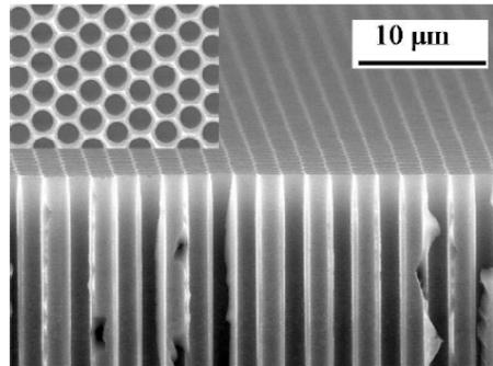
**Figure 7.** SEM image of the macroporous silicon PBG structure, produced by electrochemical etching of Si wafers in the HF/DMF solution (cross-section, inset shows top view). The PBG structure consists of vertical air cylinders arranged into the triangular lattice.
