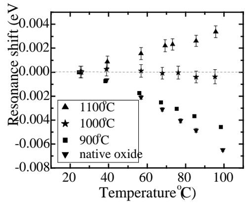
**Figure 6:** detailed experimental study of the thermal oxidation treatment needed to achieve temperature instability in 1-D PBG structures. Note that unlike in Figure 4, the porous silicon samples are made of macropores, hence the larger temperature needed.
