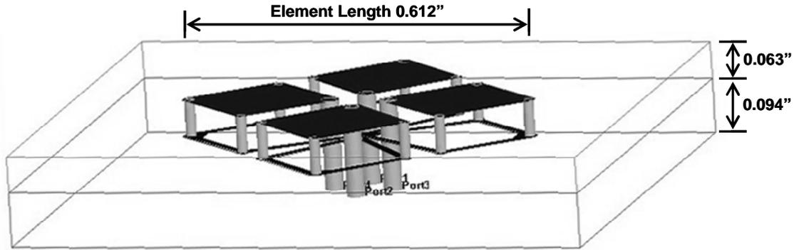
Figure 1. 3D View of One Radiating Element
