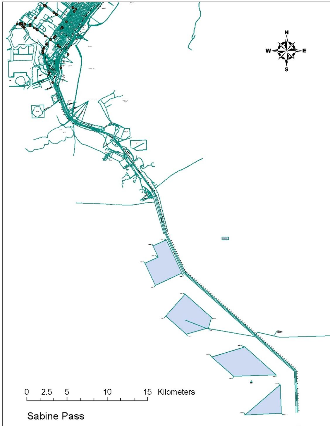
Figure 7. Project features for Sabine waterway. Sabine Lake and inland channels are north of this figure. The polygons show offshore disposal sites. The street grid at top of figure is Port Arthur.
