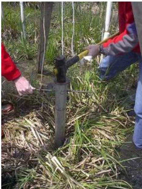
**Figure 5. Driving aluminum tube into wetland soil**
