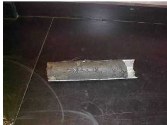
**Figure 8. Exposed soil sample from separated aluminum tube halves**
