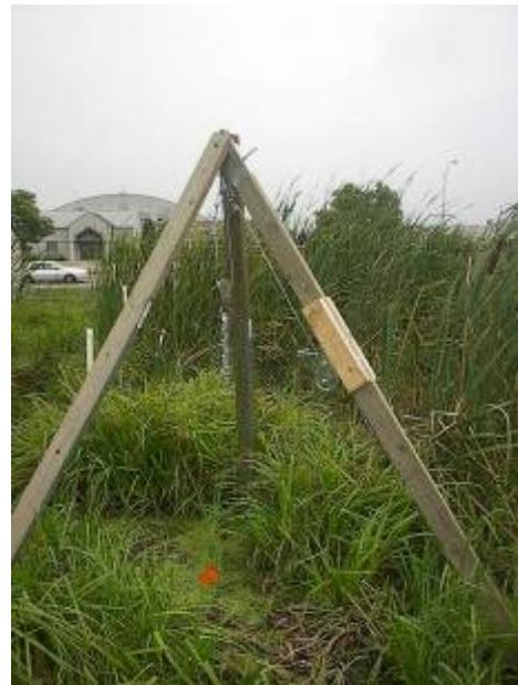
**Figure 6. Pulley on tripod mount used to extract aluminum tube from wetland soil**
