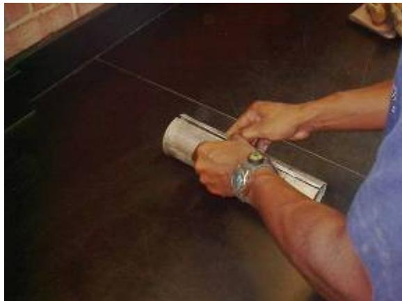
**Figure 7. Prying apart aluminum tube sections to extract soil**
