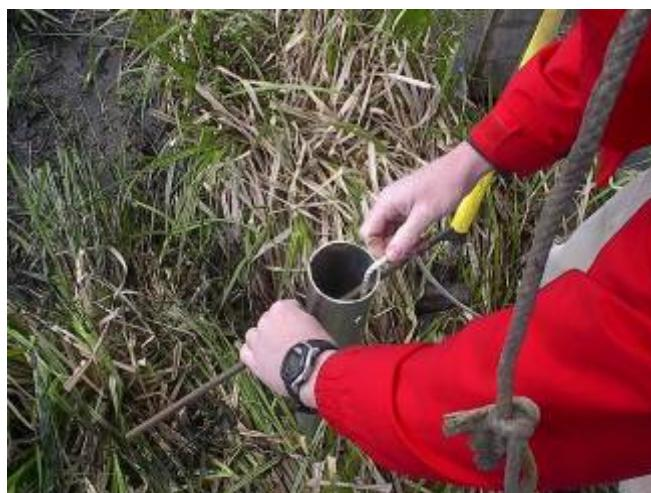
**Figure 4. Feeding plunger rope through wall of aluminum tube**
