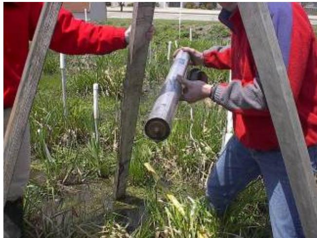
**Figure 3. Aluminum tube used for soil extraction showing rubber plunger insert**
