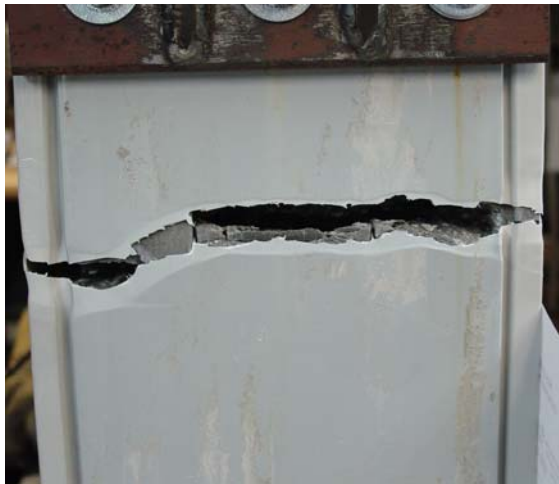
(a) Failure @ 0.003 in/sec Stroke Rate
