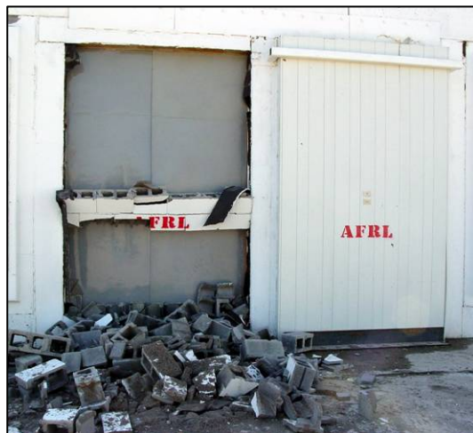
Figure 17: Experiment 3 Post-Detonation (8" Form Sand/Gravel Filled)
