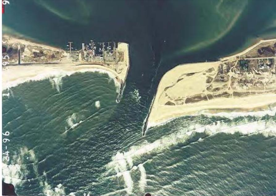
Figure 98. Shinnecock Inlet, NY, showing severely eroded downdrift beach adjacent to downdrift jetty
