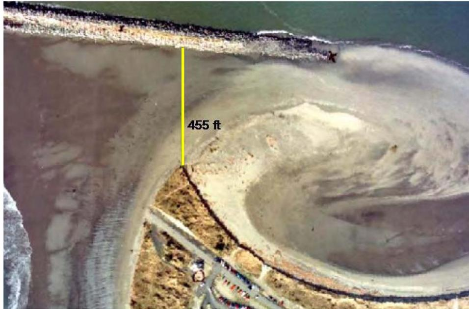
Figure A3. Breach, 6 March 1994, tide elevation +1.3 ft mllw
