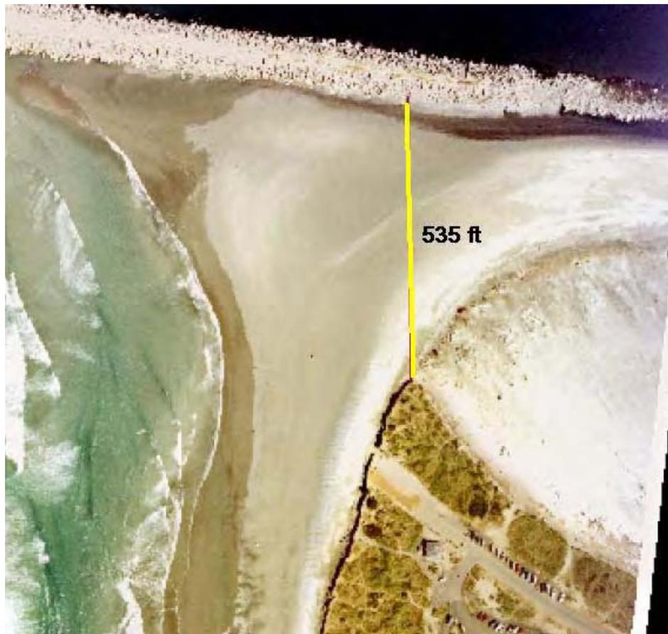
Figure A4. Breach, 10 August 1994, tide elevation +2.3 ft mllw
