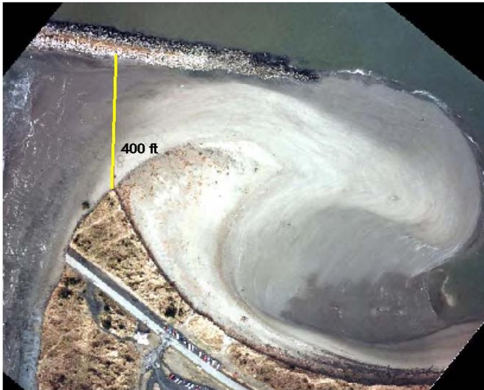
Figure A2. Breach, 2 February 1994, tide elevation +2.0 ft mllw
