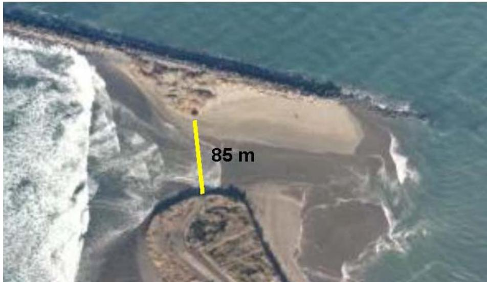
Figure 18. Breach, 17 December 1993; tide elevation +2.0 m mllw
