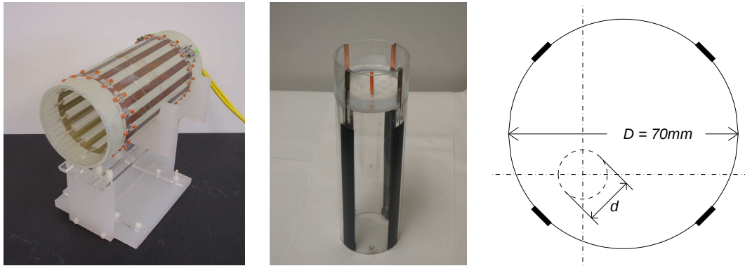
Figure 3. (a) Home-built RF coil (b) Phantom (c) Phantom description
