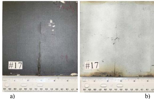
Fig. 19. Impacted cross-ply composite plates at  $I=50$  A ,  $T=158$  °F , non-perforation (test #CP-17): a) front side; b) back side.
