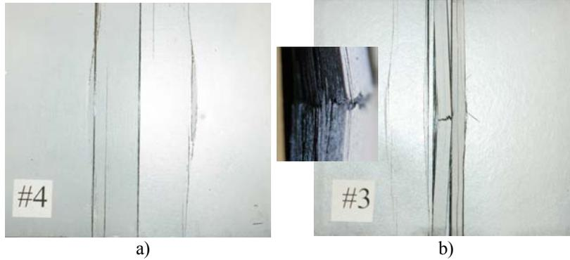
Fig. 10. Impacted unidirectional composite plates: a) test #UD-4, T=69.3 F; b) test #UD-3, T=96.7 F
