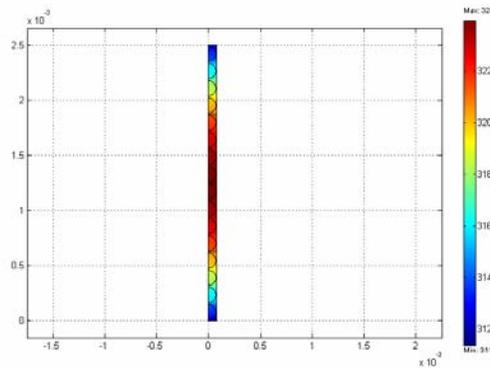
Figure 1. Temperature profile across the composite plate thickness.
