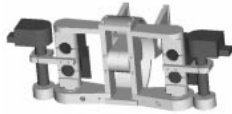
Figure 5: Rendering of the desktop active vision system produced from the engineering drawings of Figure 4.
