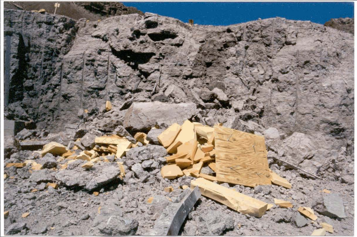
Figure 16. Test 3, Shot 2, resulting damage to Panel 3.
