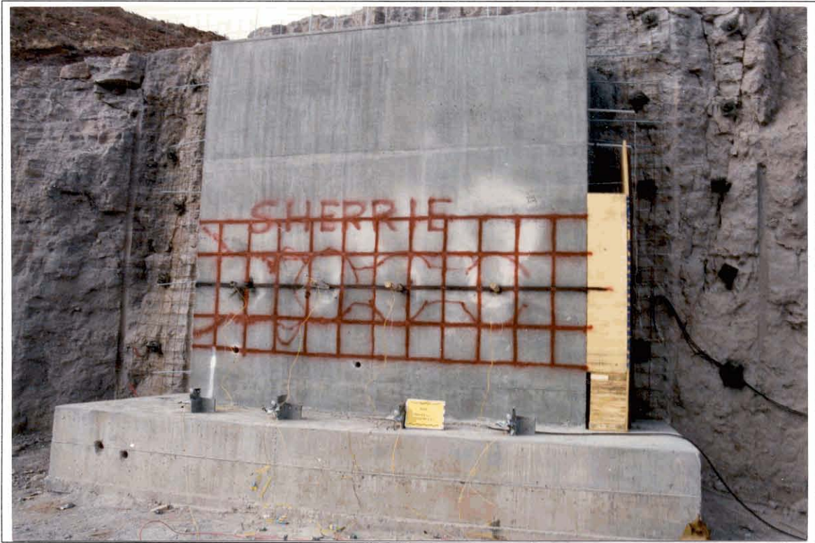
Figure 3. Panel 1 explosive charge placement.
