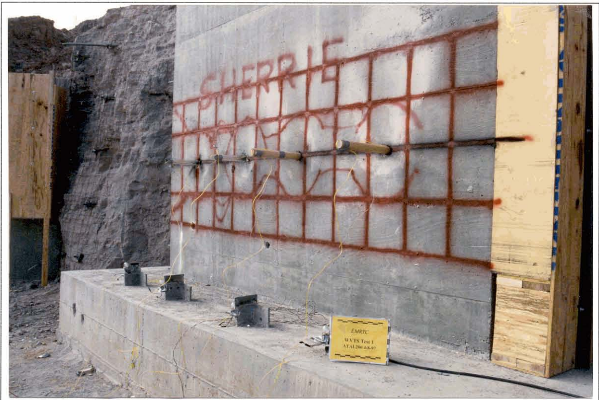
Figure 4. Panel 1 explosive charge placement.
