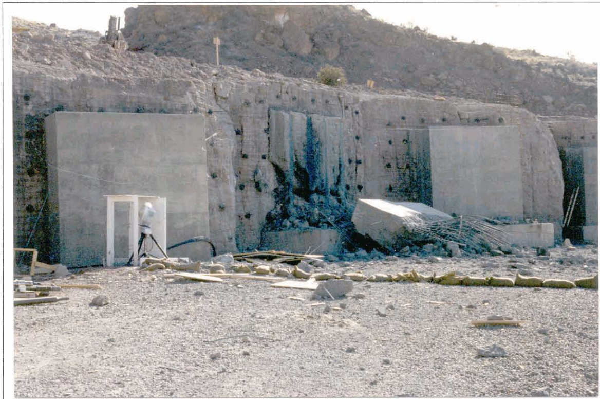
Figure 5. Test 1, resulting damage to Panel 1.
