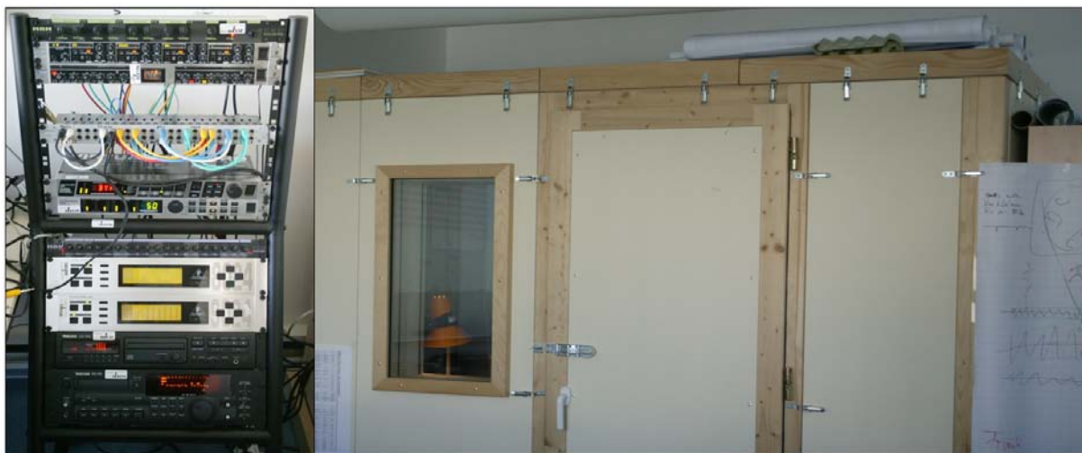
Figure 6: The anechoic chamber with its connection and control panel.
