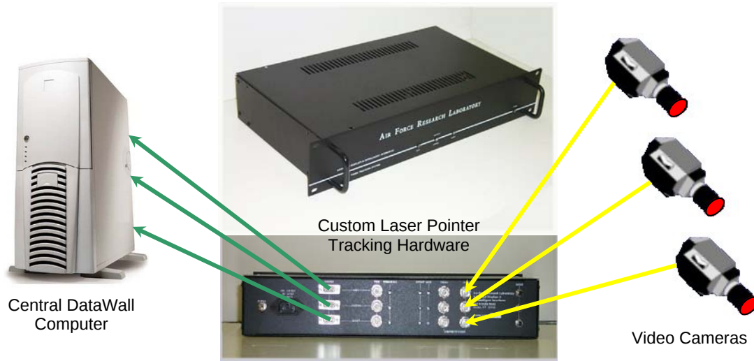
Figure 14 AFRL/IF's Custom Laser Pointer Tracking Subsystem Architecture
