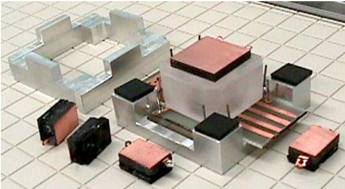
Fig. 36 — Parts assembly for the Compact device
