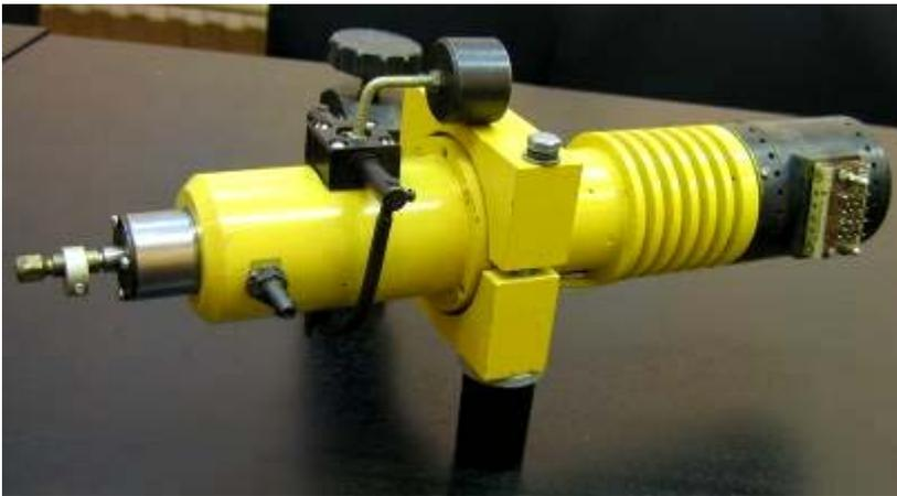
Fig.16 Tool with rotating electrode for mechanization of deposition process of coating.
