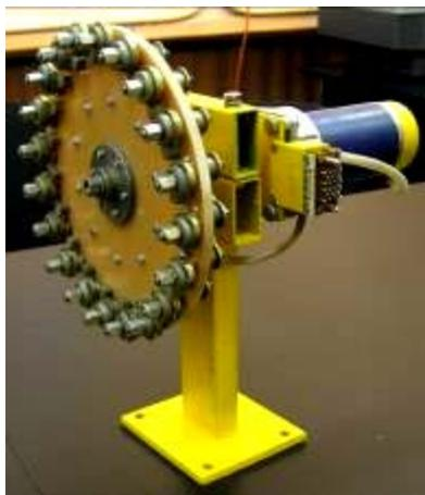
Fig.17 Multi-electrodes tool for mechanization of deposition process of coating.
