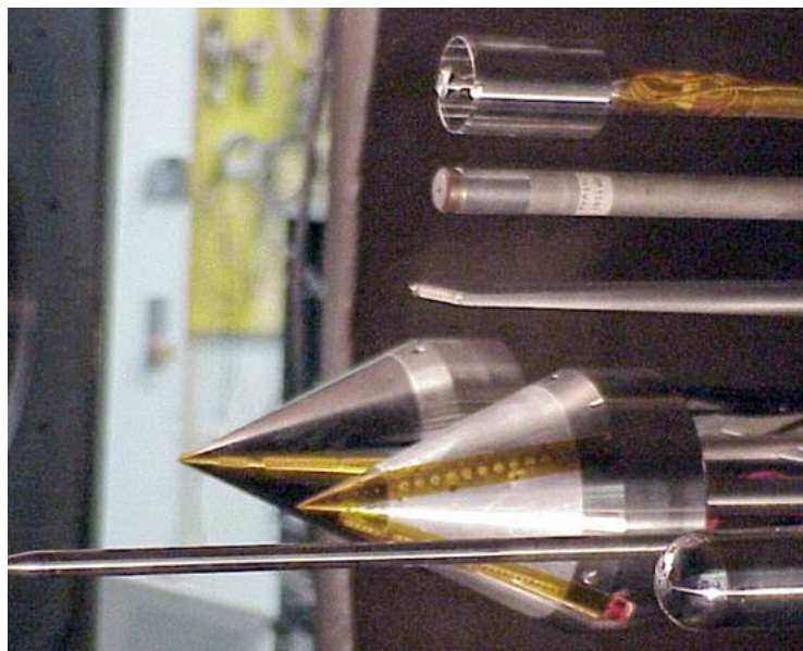
Figure 11: Two 25° Cone Models in Survey Rake for “Vibrational Nonequilibrium” Studies.
