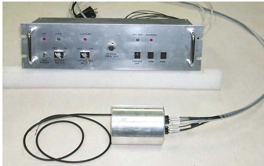
Figure 8 Photograph of Controller and Firing Set
