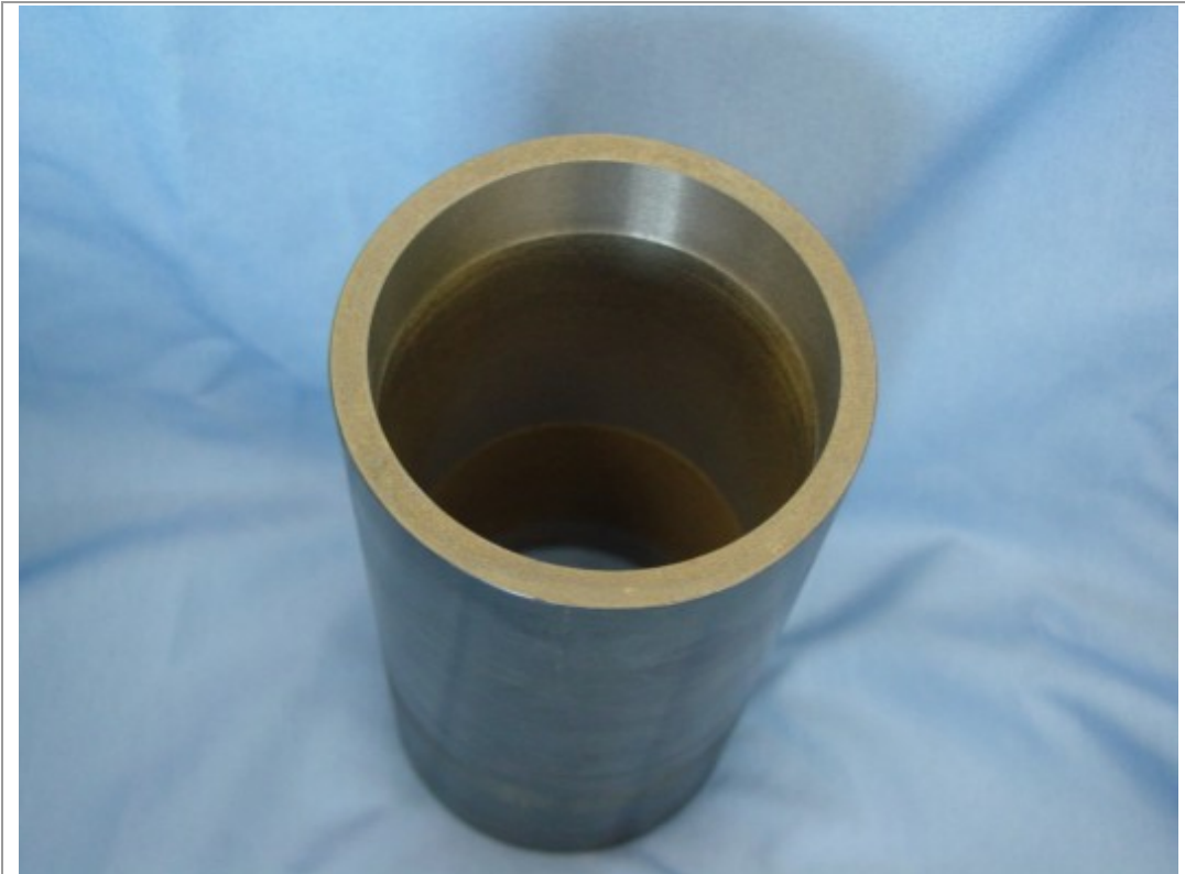
Figure 6-1 3" ID cylinder sprayed with WC self fluxing coating (Ni-988) and ground at end to 12-16 \mu " Ra.
