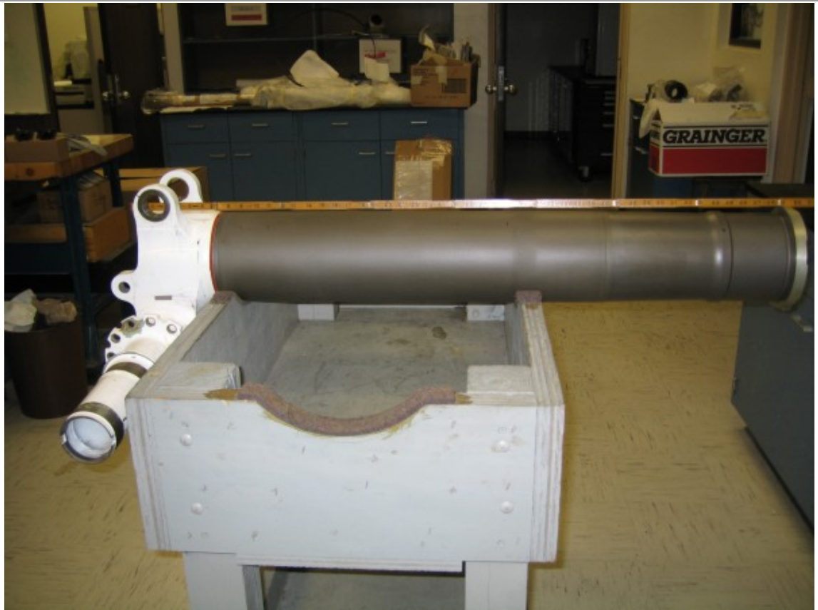
Figure 8-1 P-3 landing gear inner cylinder after Lockheed-Martin rig test (HVOF coating stripped from OD – ID usually chrome plated).
