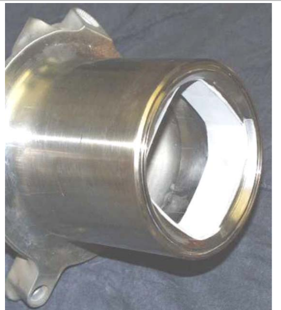
Figure 1-2 CF-18 A/B axle polygon HVOF sprayed from outside (Messier-Dowty).
