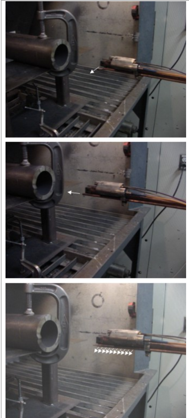
Figure 5-5 Sparging gas arrangements for ID plasma spray. Top – side on; middle – end on; bottom – line.
