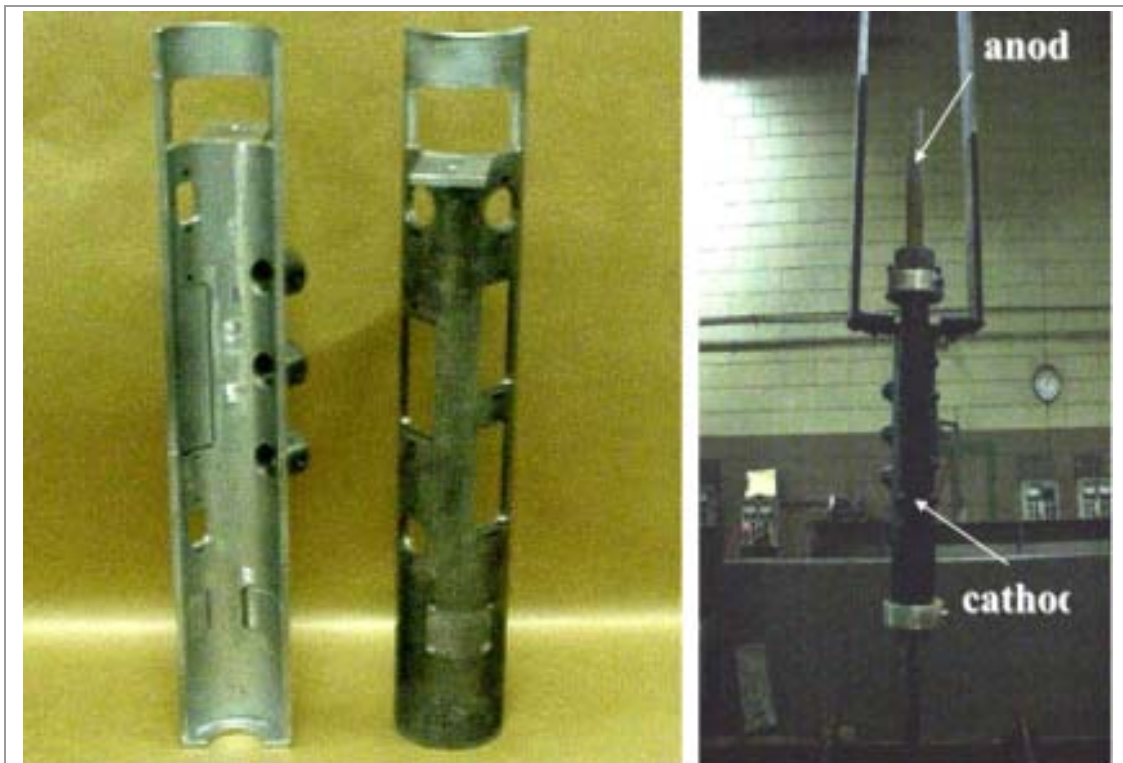
Figure 4-2 Hard chrome electroplating arrangement.
