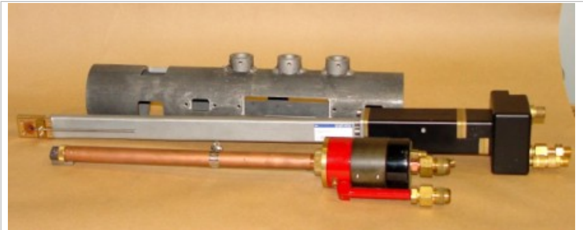
Figure 2-2 Praxair SG-2700 gun (front) and Sulzer Metco F-210 gun (center) in front of the 3” ID, 18” long sample holder (back).
