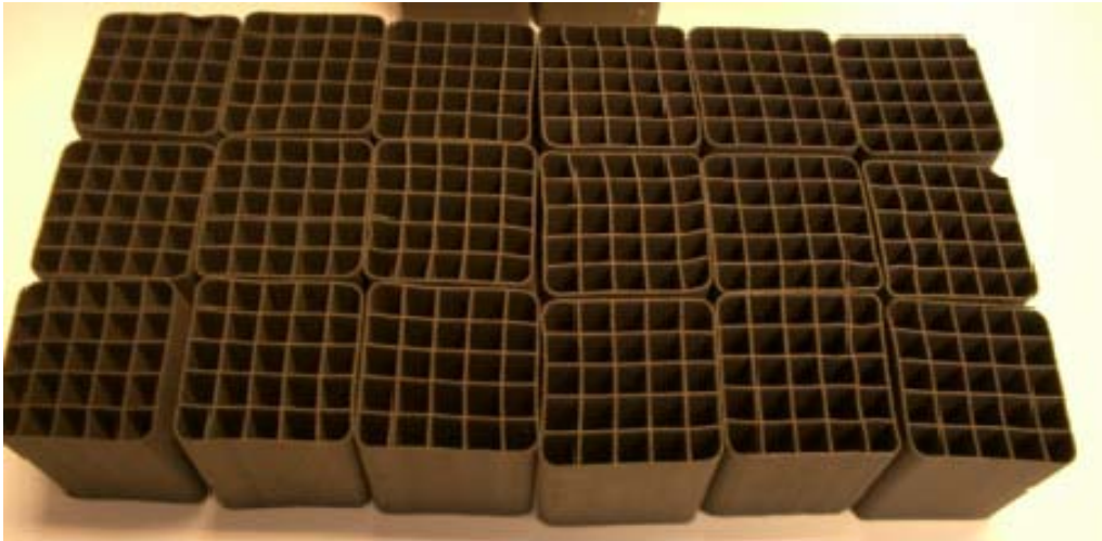
As-extruded dimensions – 1.3" x 1.3" x 1.3"
