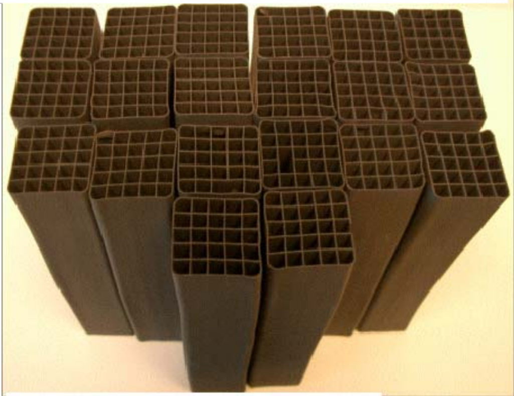
As-extruded dimensions – 1.3" x 1.3" x 7.0"
