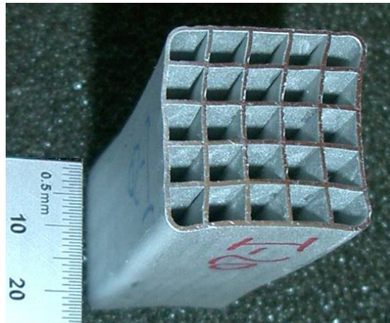
Figure 1. Super Invar, square cell LCA with a cell size of 0.19 inches and a relative density of 20%.
