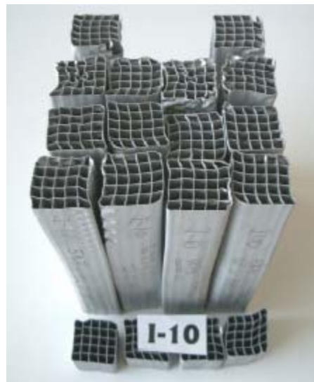
Figure 15. Final Super Invar LCAs delivered to ARL at 10, 15, and 20% relative density.
