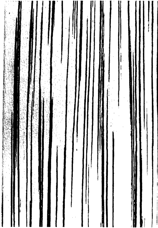
(b) Longitudinal section. Unetched; x150.
