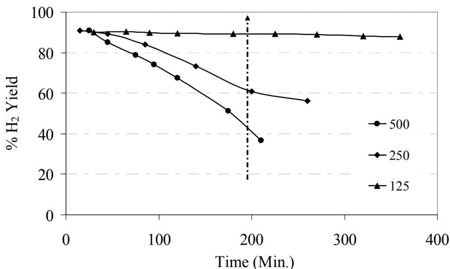
**Figure 9: Hydrogen yield vs. time at different benzothiophene concentrations (125 – 500 ppmw) at the optimal conditions of  $S/C = 0.71$ ,  $O_2/C = 0.36$ ,  $GHSV = 4500\text{hr}^{-1}$ ,  $T = 885^\circ\text{C}$ , and  $P = 1\text{bar}$**
