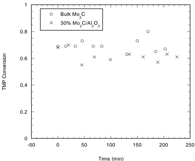
**Fig 10: Comparison of bulk and supported catalysts for TMP steam reforming.**
