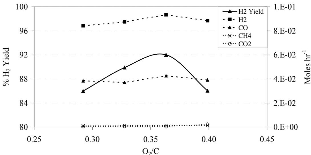
**Figure 6: Hydrogen yield and molar flow rate of the products as a function of  $O_2/C$  ratio during OSR of hexadecane over a bulk  $Mo_2C$  catalyst at a temperature of 885°C,  $S/C$  of 0.71,  $P=1bar$ , and  $GHSV$  of 3500  $hr^{-1}$ .**
