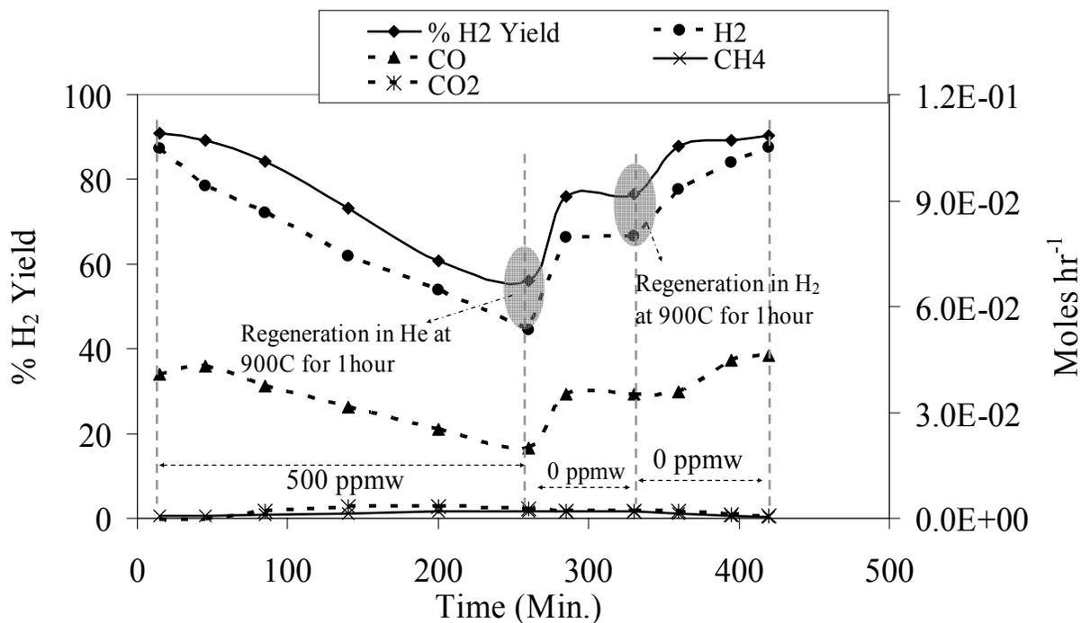
**Figure 8: Hydrogen yield and products composition as a function of time during hexadecane oxidative-steam reforming experiments in presence of 500 ppmw of benzothiophene at the optimal conditions of  $S/C = 0.71$ ,  $O_2/C = 0.36$ ,  $GHSV = 4500\text{hr}^{-1}$ ,  $T = 885^\circ\text{C}$ , and  $P = 1\text{bar}$ .**
