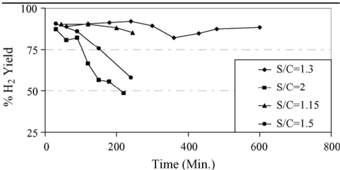
**Fig. 1. Long-term catalytic activity of Mo<sub>2</sub>C for TMP steam reforming at a temperature of 1000 °C and GHSV of 1500 h<sup>-1</sup>.**
