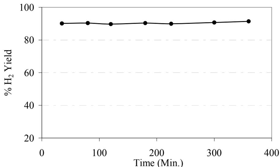
**Figure 7: Long-term performance (H<sub>2</sub> yield) of bulk Mo<sub>2</sub>C for OSR of hexadecane at the optimal conditions of S/C=0.71, O<sub>2</sub>/C=0.36, GHSV=4500hr<sup>-1</sup> and T=885°C, P=1bar.**
