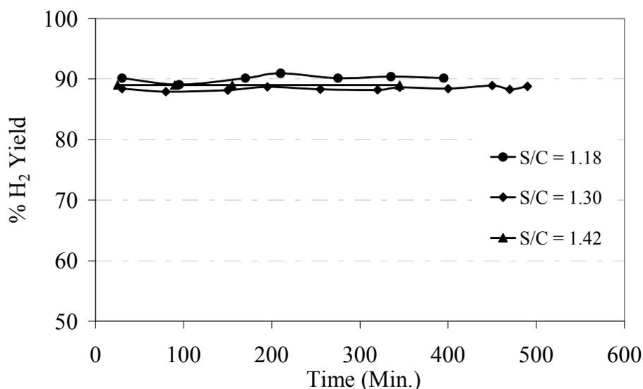
**Figure 5: Long-term performance ( $\text{H}_2$  yield) of bulk  $\text{Mo}_2\text{C}$  for SR of hexadecane at different S/C ratios at  $T = 965^\circ\text{C}$ ,  $P=1\text{bar}$ , and  $\text{GHSV} = 5500\text{ hr}^{-1}$ .**
