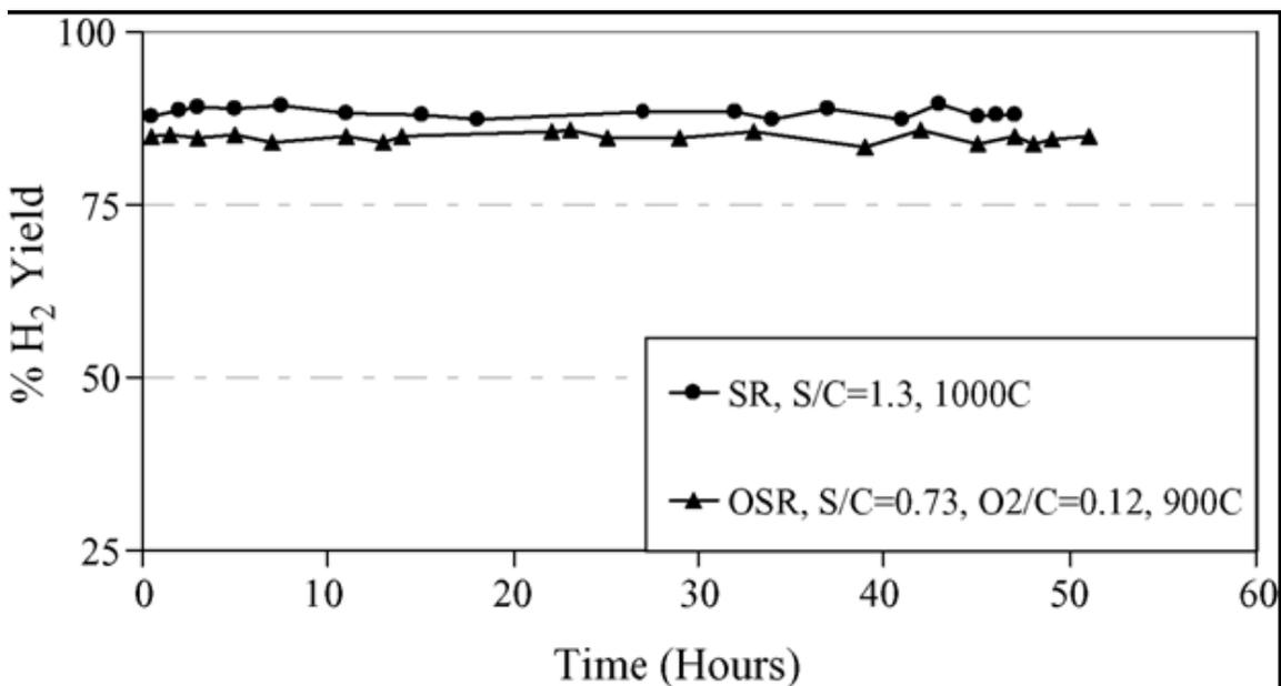
**Fig 2. Long term catalytic stability for steam and oxidative steam reforming of TMP. GHSV = 1500 h<sup>-1</sup>**
