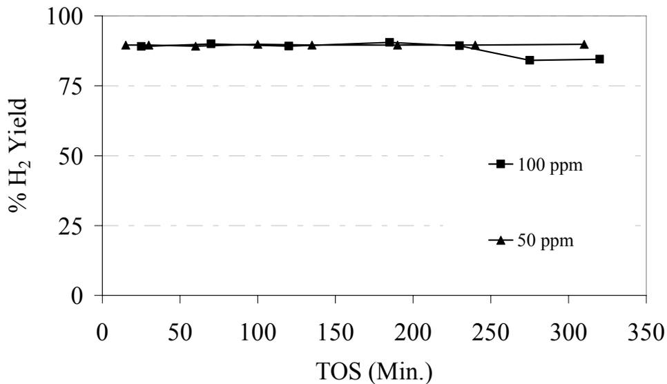
**Figure 4: Hydrogen yield during OSR at low thiophene concentrations. S/C=0.73, O<sub>2</sub>/C=0.12 & T=900 C**
