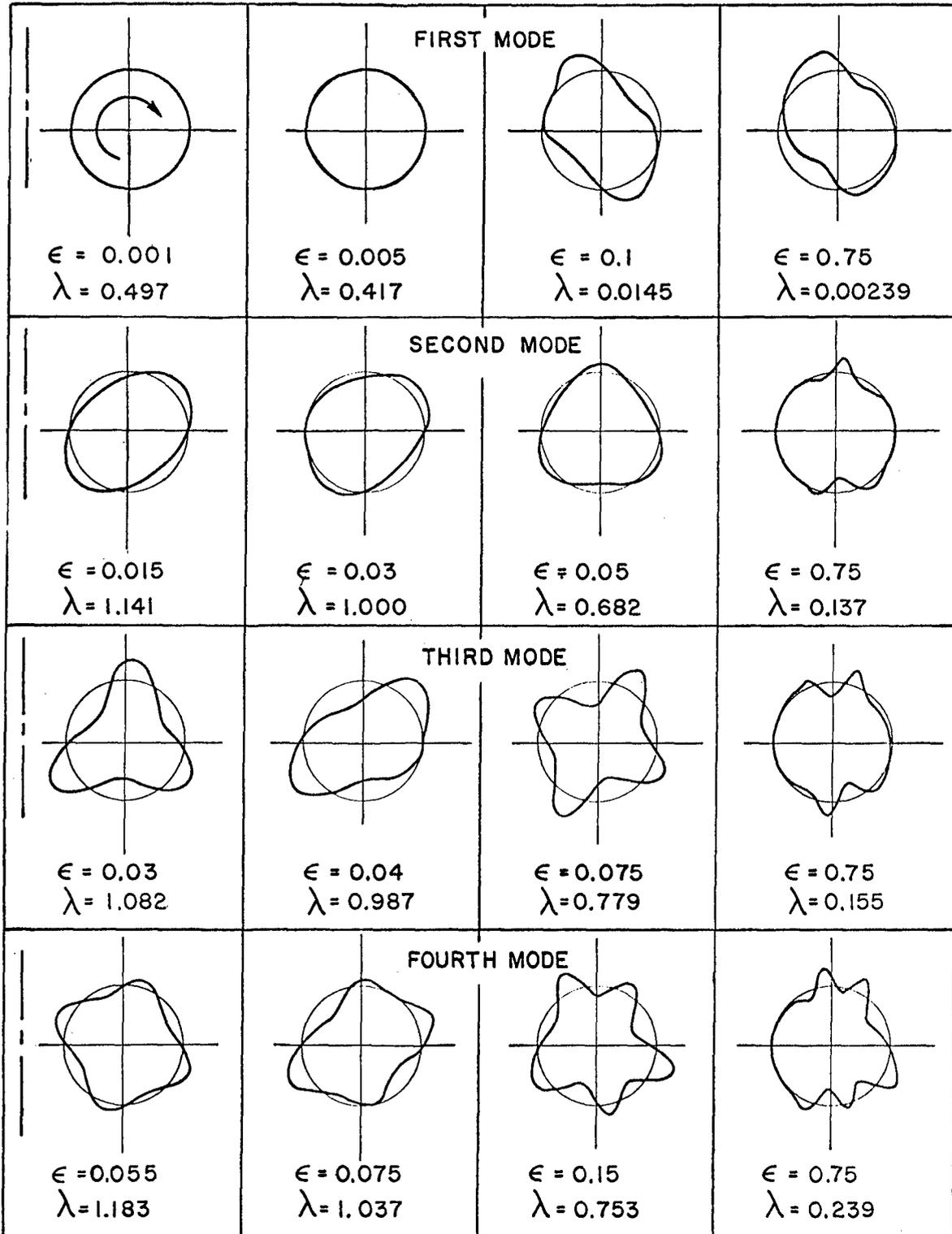
FIG. 15: AXISYMMETRIC MODE SHAPES, ANTISYMMETRIC,  $K=0$ ,  $h/R=0.01$
