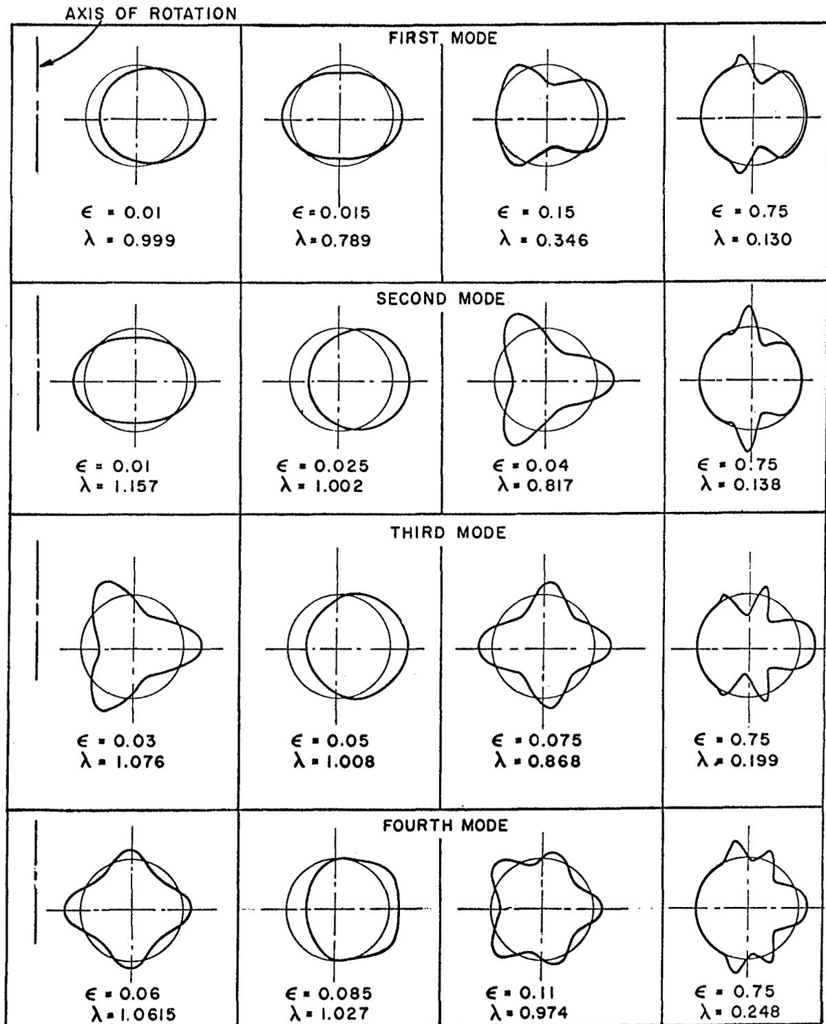
FIG.14: AXISYMMETRIC MODE SHAPES, SYMMETRIC,  $\kappa=0$ ,  $h/R=0.01$
