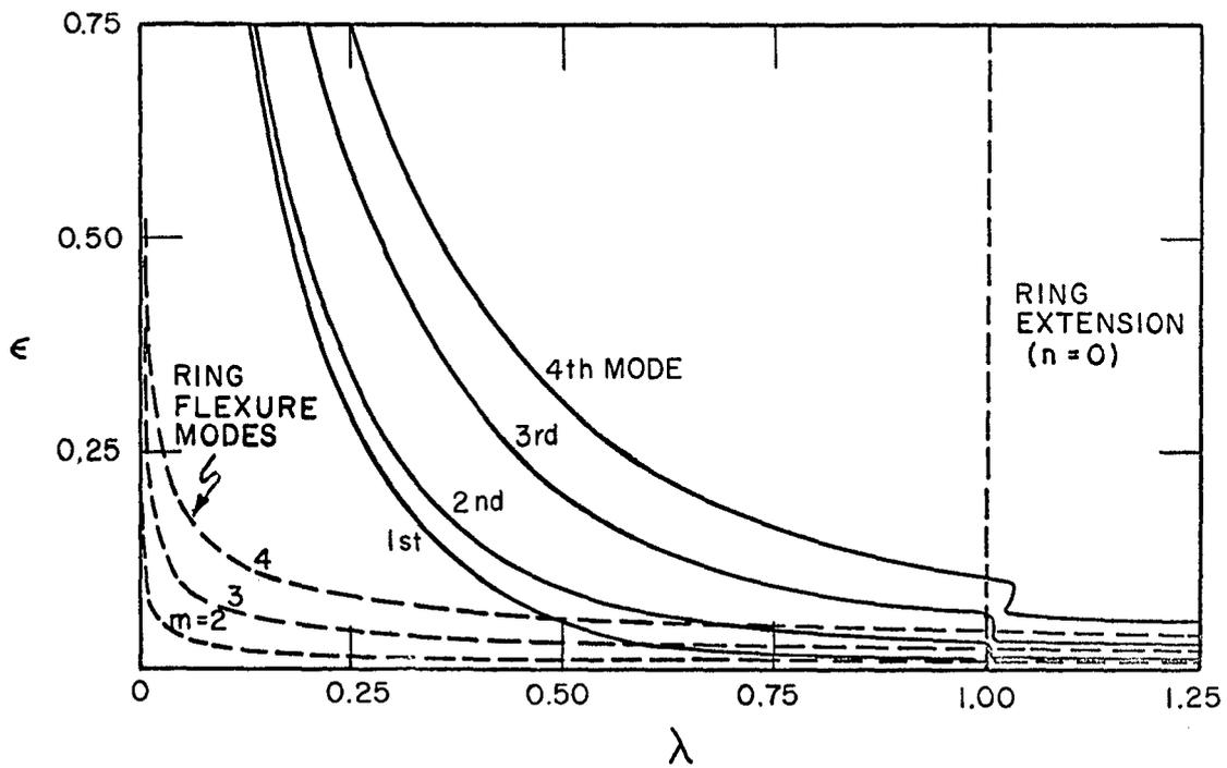
FIG. 10: AXISYMMETRIC MODES, SYMMETRIC,  $K = 0, h/R = 0.01$
