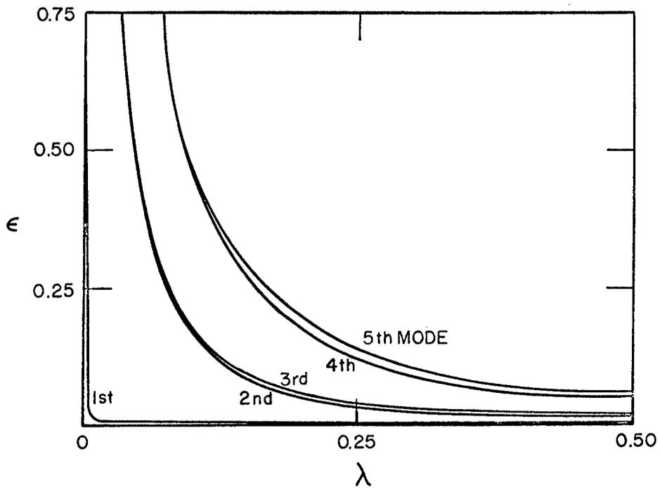
FIG. 17: AXISYMMETRIC MODES, ANTISYMMETRIC,  $\kappa=0, h/R=0.001$
