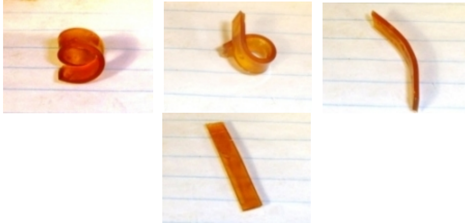
Figure 6: Cyanate ester shape memory polymer exhibiting shape recovery from deformed configuration (left) to memorized configuration (right) when activated by heat
