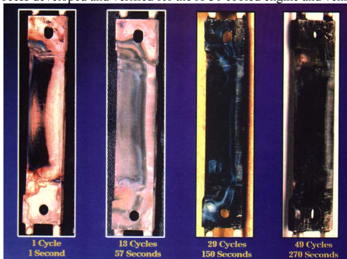
Figure 13: Test of engine heat exchangers and leading edges (Ref. U17)
