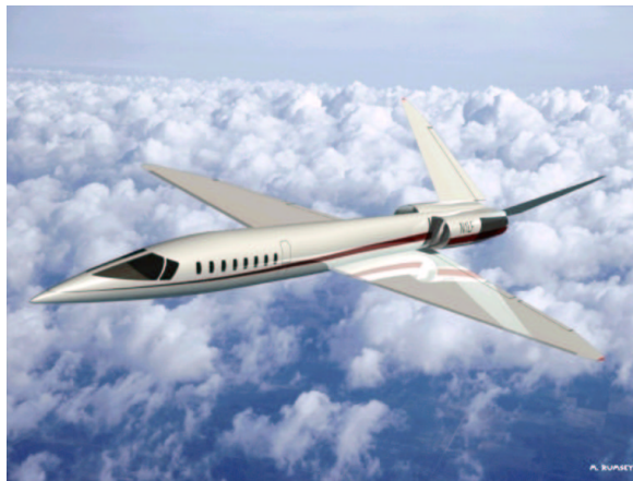
Fig. 2 Natural laminar flow supersonic business jet configuration.
