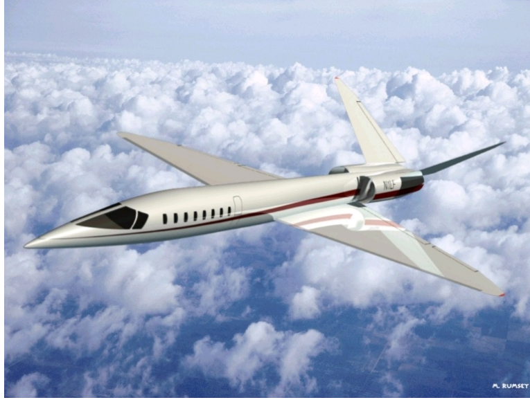
Figure 5-1: Natural laminar flow supersonic business jet configuration.
