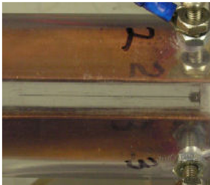
Figure 4. Corona needle inserted into quadrupole.
