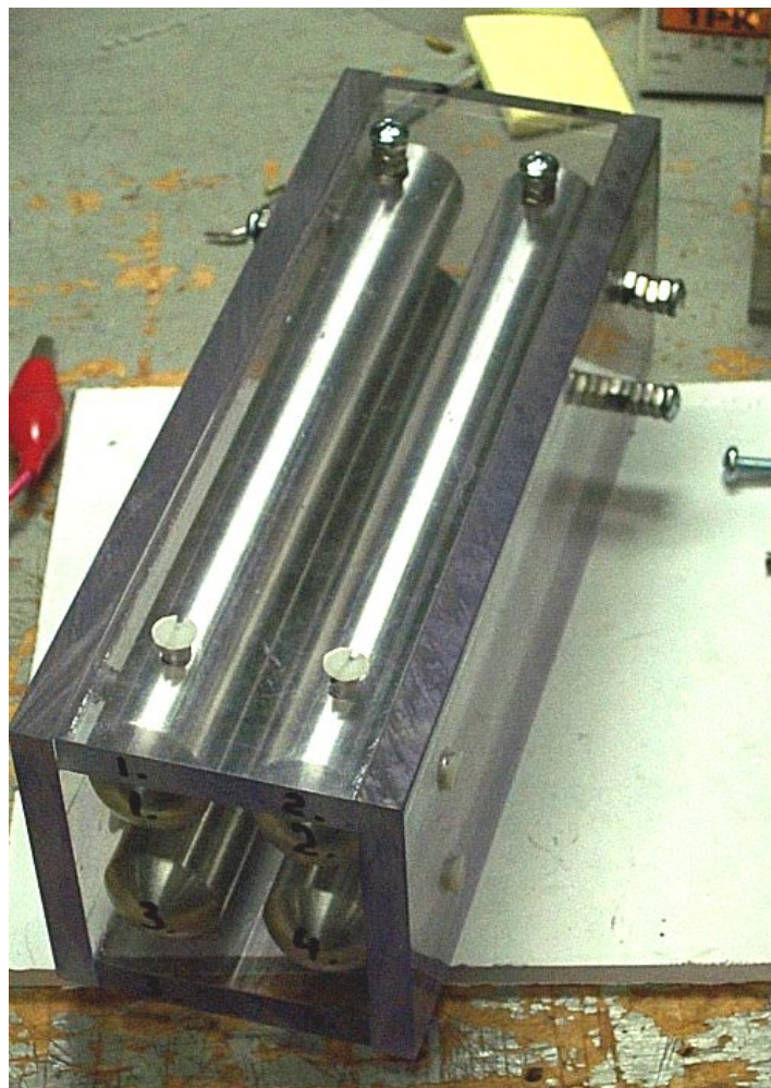
Figure 7. Second quadrupole built with 2.54 cm diameter rods.
