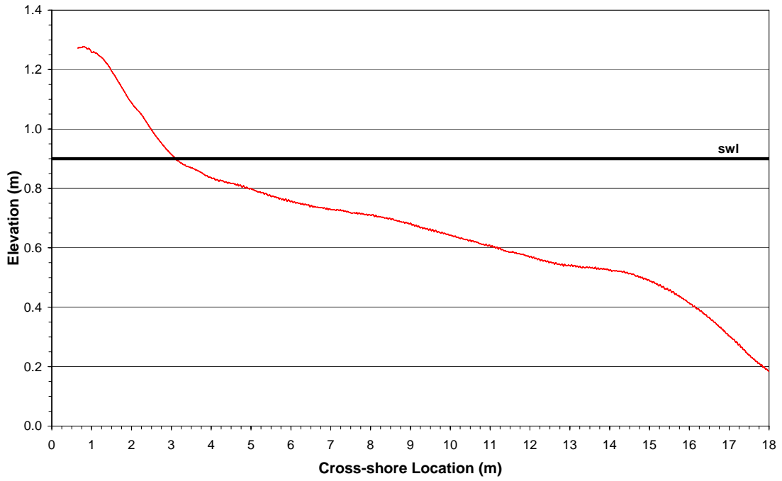
Figure 4-2. Quasi-equilibrium beach profile formed from Test 1 waves
