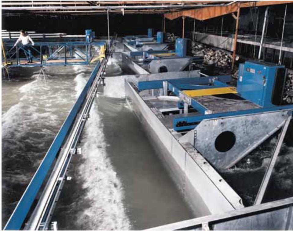
Figure 3-3. LSTF wave generators
