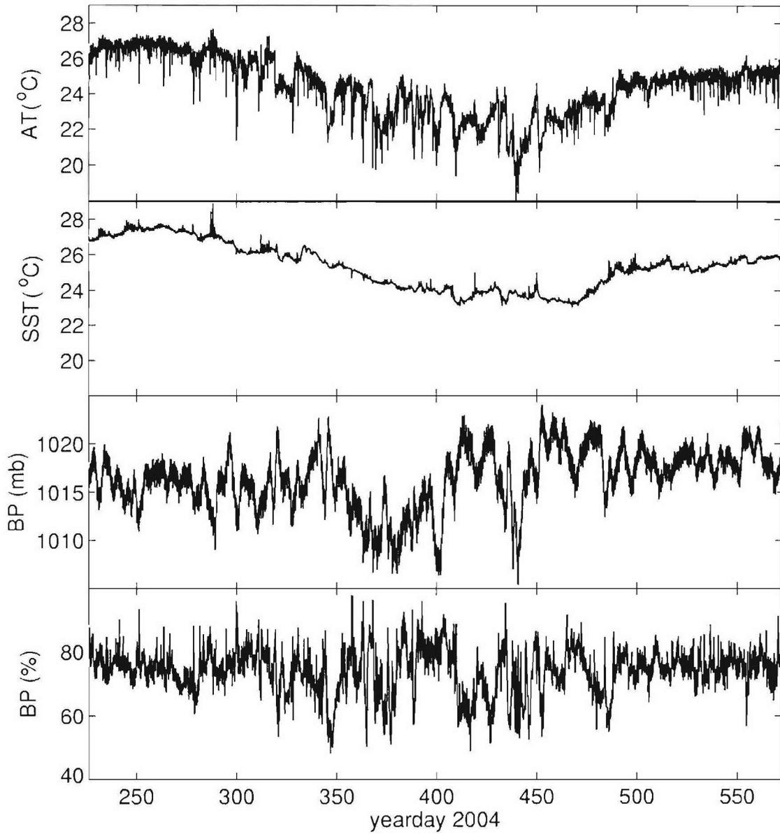
**Figure 8. WHOTS-1 meteorological variables: Part 1. Raw data from ASIMET System 1 (black) and System 2 (gray) averaged to 1 hour are plotted. Variables shown from top to bottom are: Air temperature (AT, °C), sea surface temperature (SST, °C), barometric pressure (BP, mb) and relative humidity (RH, %).**
