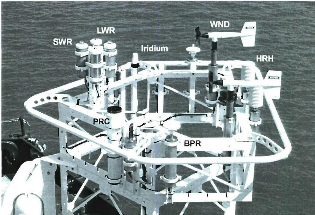
Figure 17. The WHOTS-2 tower top on the deck of the *Melville* with ASIMET modules labeled. When deployed, the windward side of the buoy is to the right and the wind vanes point in the opposite direction. The GPS module is to the right of the Iridium antenna on the far side of the tower. The sea surface temperature and conductivity (STC) modules, located on the underside of the buoy, are not visible in this view.
