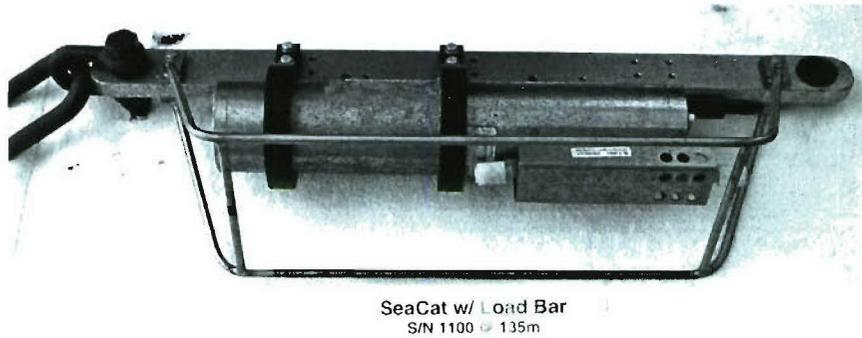
Figure 11. WHOTS-1 SeaCAT from 135 depth. The instrument is clamped to a load bar, which is shackled in-line with the mooring.
