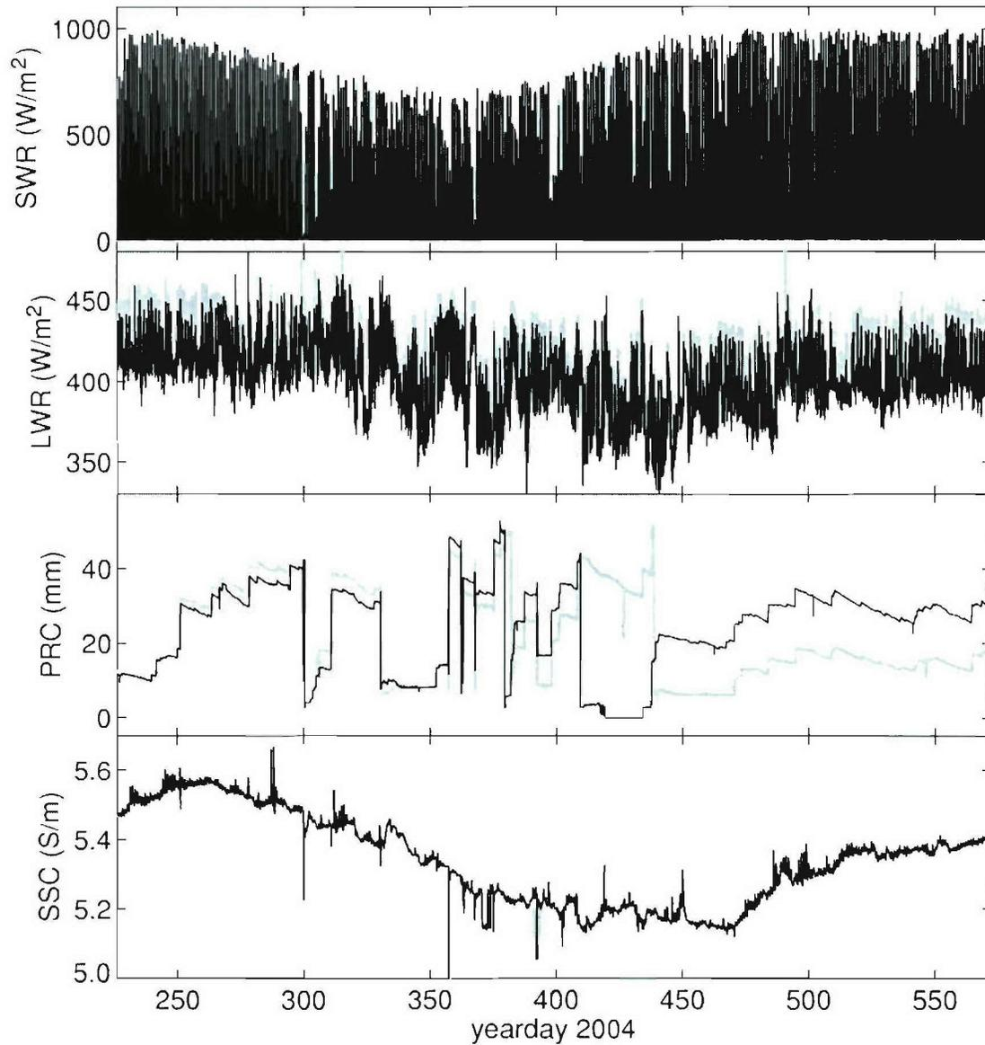
**Figure 9. WHOTS-1 meteorological variables: Part 2. Raw data from ASIMET System 1 (black) and System 2 (gray) averaged to 1 hour are plotted. Variables shown from top to bottom are: shortwave radiation (SWR,  $\text{W}/\text{m}^2$ ), longwave radiation (LWR,  $\text{W}/\text{m}^2$ ), precipitation level (PRC, mm) and conductivity (COND,  $\text{mS}/\text{m}$ ).**
