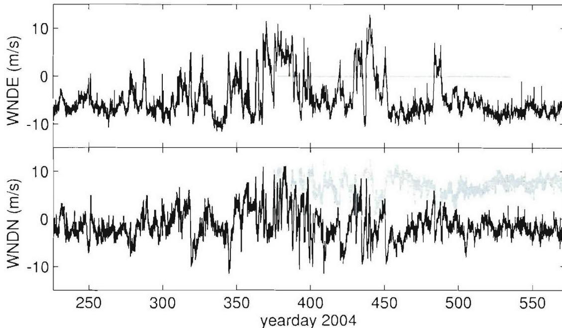
**Figure 10. WHOTS-1 meteorological variables: Part 3. Raw data from ASIMET System 1 (gray) and System 2 (black) averaged to 1 hr intervals are plotted. Variables shown from top to bottom are: east wind component (WND-E, m/s), north wind component (WND-N, m/s). Directions are in “oceanographic” convention– direction towards.**
