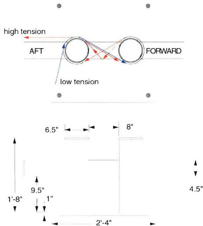
**Figure 21. H-Bit dimensions and fair lead detail.**
