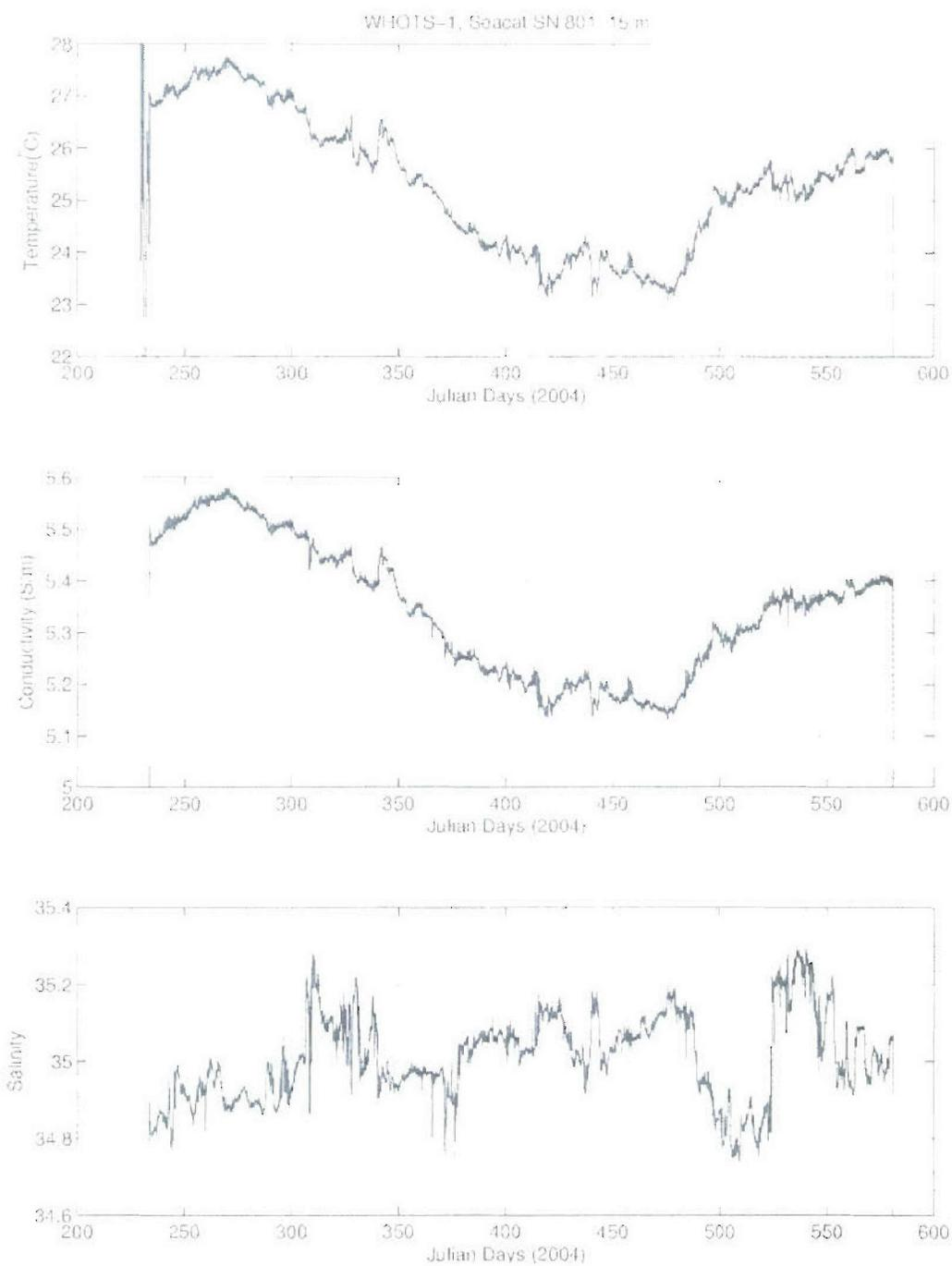
**Figure 14. Temperature (upper panel), conductivity (middle) and salinity (lower) from WHOTS-1 SeaCAT SN 0801 deployed at 15 m.**
