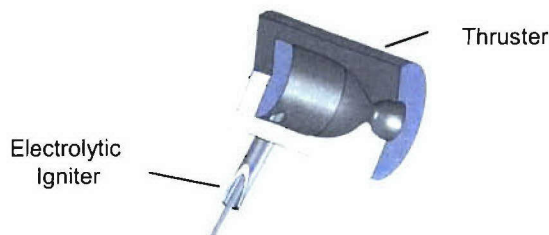
Figure 3. Thruster body with electrolytic igniter.
