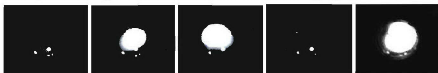
Figure 10. The flame oscillation sequence in the vortex combustor. The mass flow rate of nitromethane was 0.0127 g/s.
