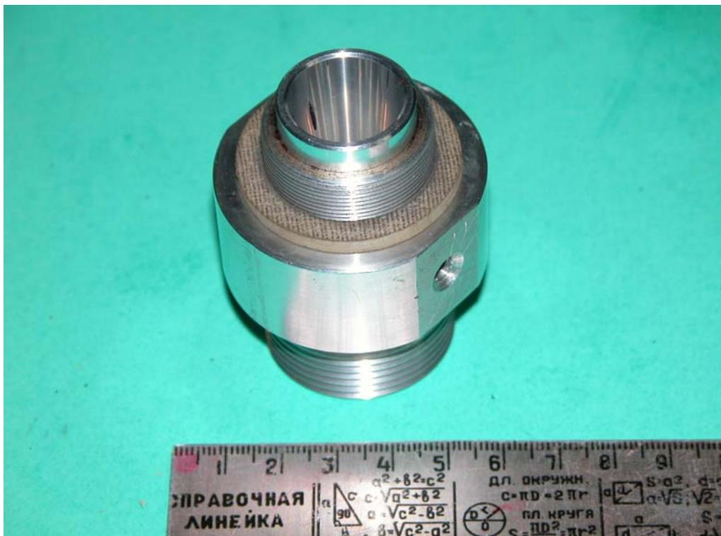
Fig.2.7. Nozzle with pointwise feeding of the liquid (test section, variant 2)
