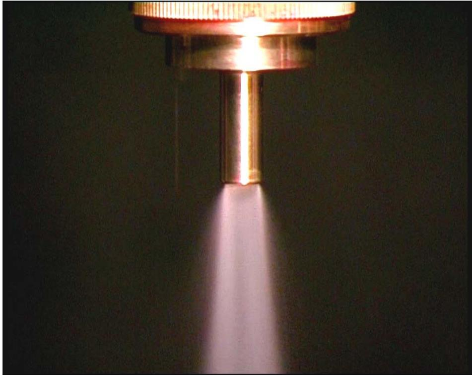
Fig. 2.44. Ejection of the liquid with a co-current gas flow into the atmosphere
