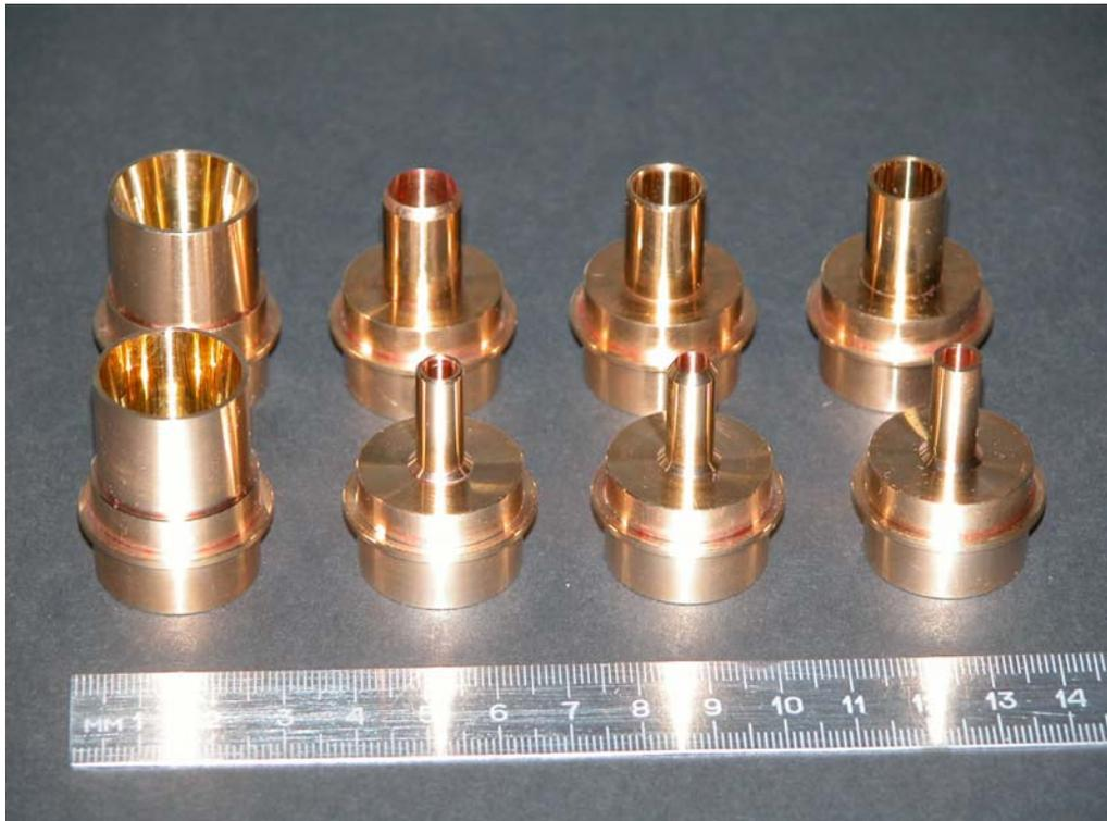
Fig. 2.6. Exchangeable exit channels
