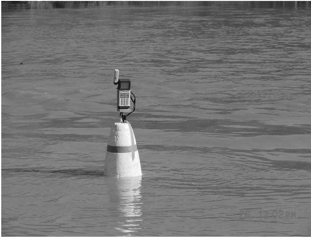
Figure 4. Float with GPS receiver mounted on top standing vertical in the water (after Winkler and Wooley 2002).
