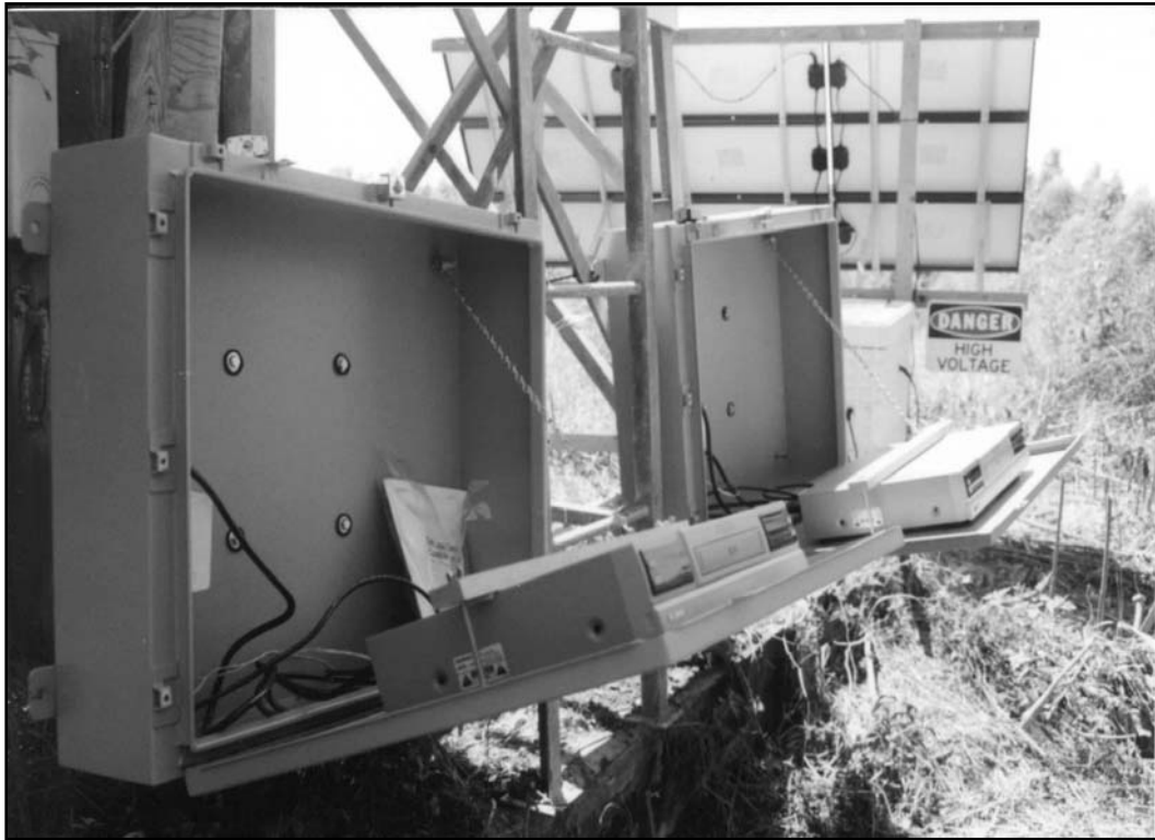
Figure 5. Time-lapse recorder and open enclosure (after Winkler et al. 2003).
