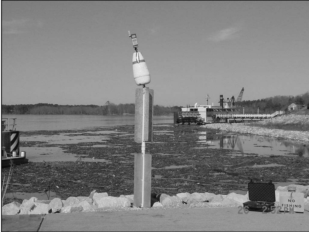
Figure 3. Float with two sections configured to draft 8 ft (after Winkler and Wooley 2002).
