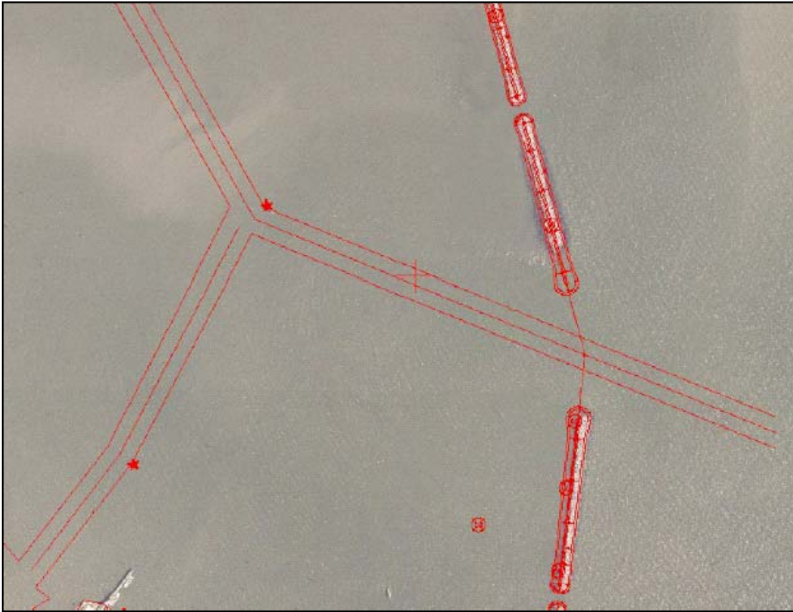
Figure A11. Schematic of existing breakwater configuration (121.9-m (400-ft) gap) versus authorized breakwater alignment (91.4-m (300-ft) gap) (red outline) with respect to channel outline, Tedious Creek, MD.
