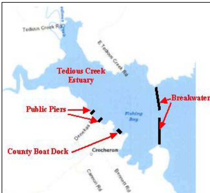
Figure 4. Location of Tedious Creek breakwater, and public piers and county boat dock on the south shore subjected to excessive wave heights during storm conditions.
