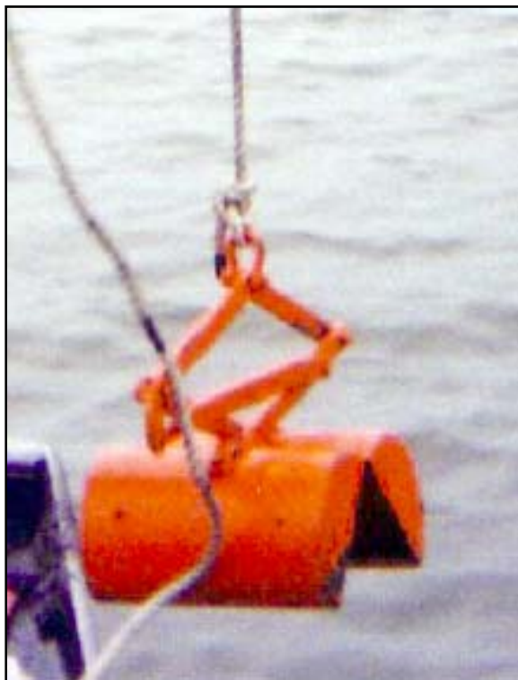
Figure 26. Clamshell bed material sampler used at Tedious Creek, MD (after Pratt 2003).
