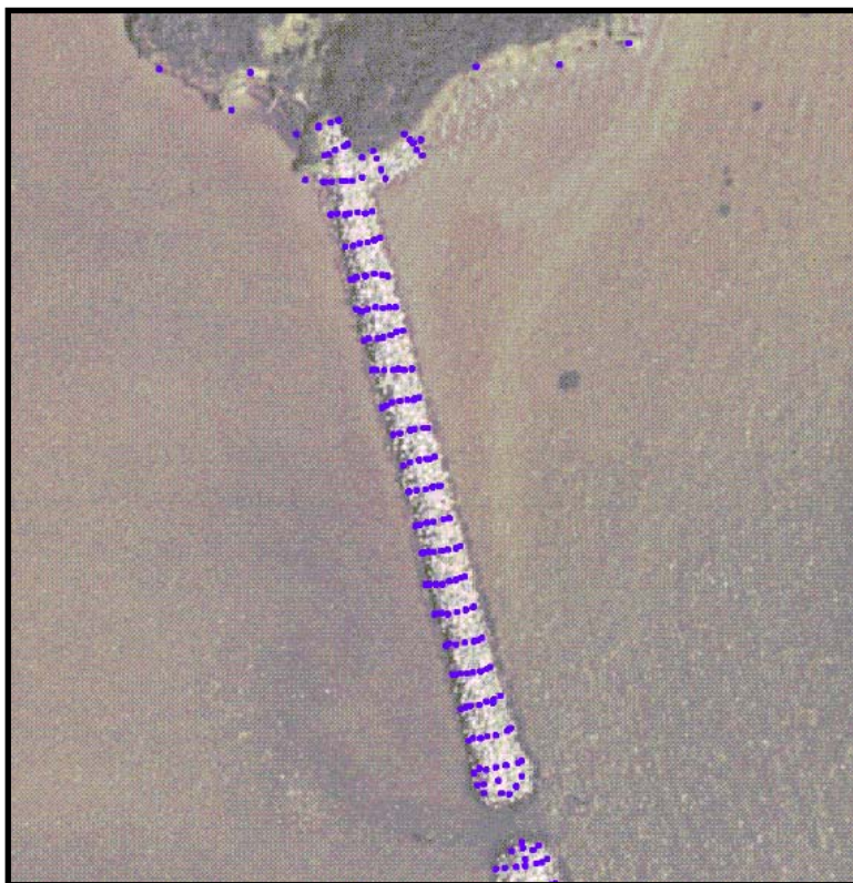
Figure 22. Breakwater cross-section survey lines, and examples of bank line delineation, Tedious Creek, MD (after Pratt 2003).
