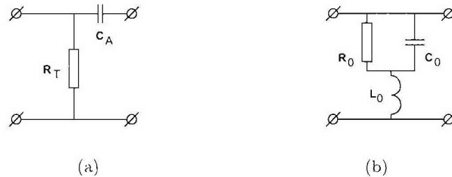
Figure 4: Circuits considered as an antenna node ( n = 0 ) or a resonant chain ( n = N_{LC} )
