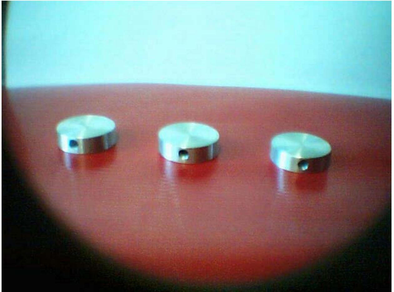
Fig. 1. Samples of aluminum alloy 2024 – T3 prepared for the MPO process.
