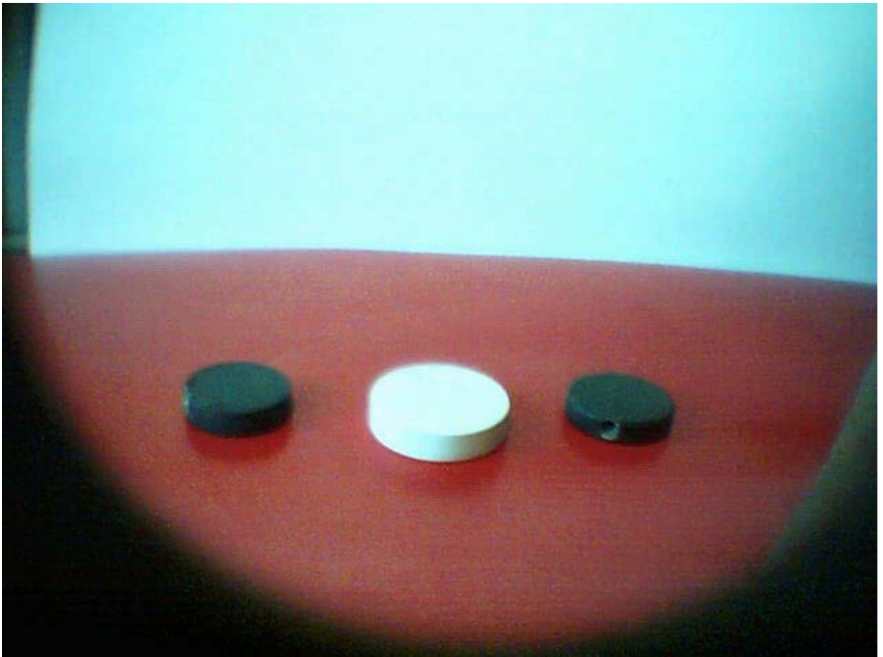
Fig.3. Views of samples of aluminum alloy 2024 – T3 after MPO processing. Black – in KOH electrolyte, white – in \text{Na}_2\text{CO}_3 electrolyte.
