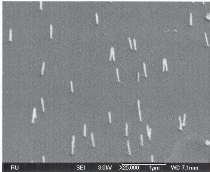
Fig. 6. SEM image (45° tilted sample) of PEC-etched MOCVD-grown n-type GaN layer (sample labeled #2190-1.1).
