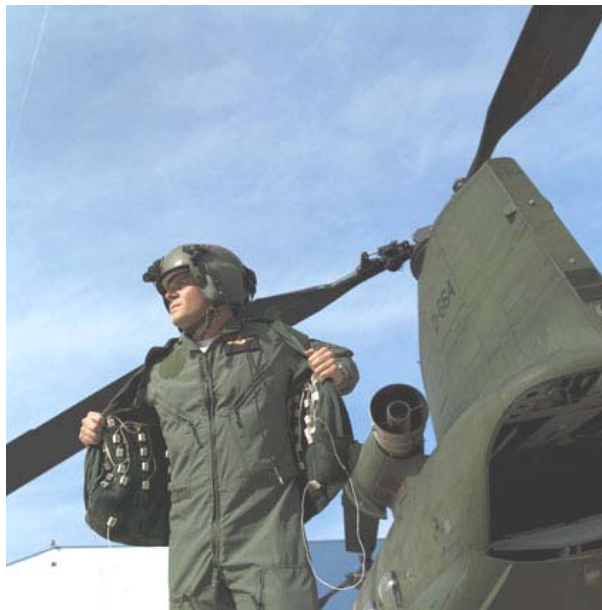
Figure 13: Pilot Wearing a Laboratory Version of the TNO Tactile Torso Display (TTTD), or Tactile Suit (in the back: a RNLAf Chinook Helicopter). This particular version of the TTTD contains twelve columns of five rows of vibro-tactile actuators, plus four more on shoulders and between the upper legs and the seat.
