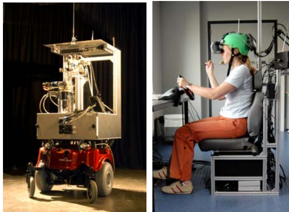
Figure 6: 'The General' Tele-Presence Enabled Unmanned Ground Vehicle (indoor version; at the left) and the Ground Control Station (at the right).
