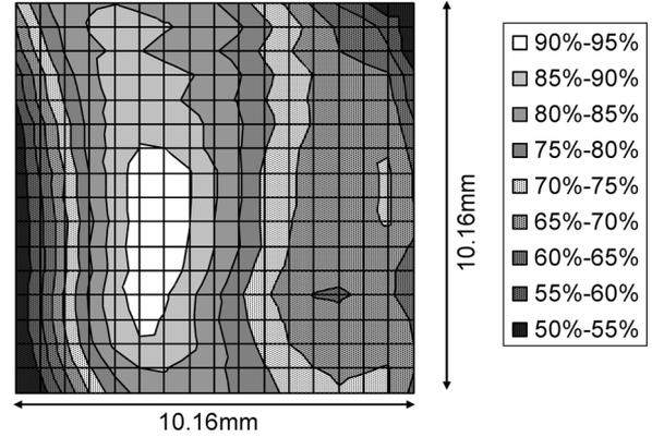
Fig. 2. Diffraction efficiency mapping of the VBG.
