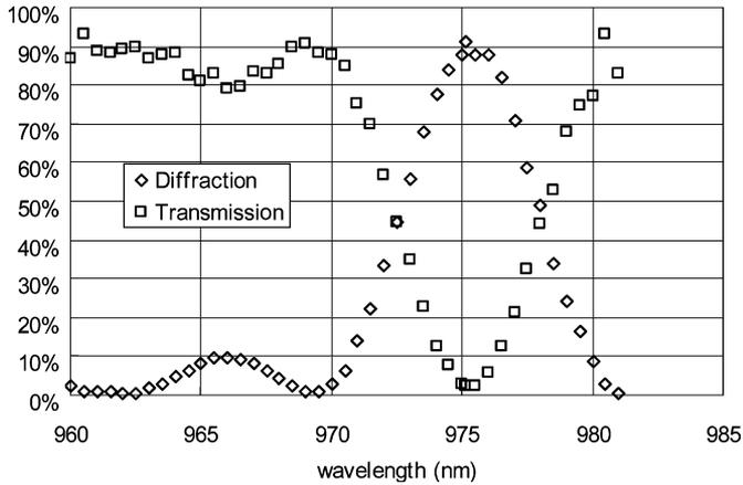
Fig. 1. Diffraction and transmission spectrum.
