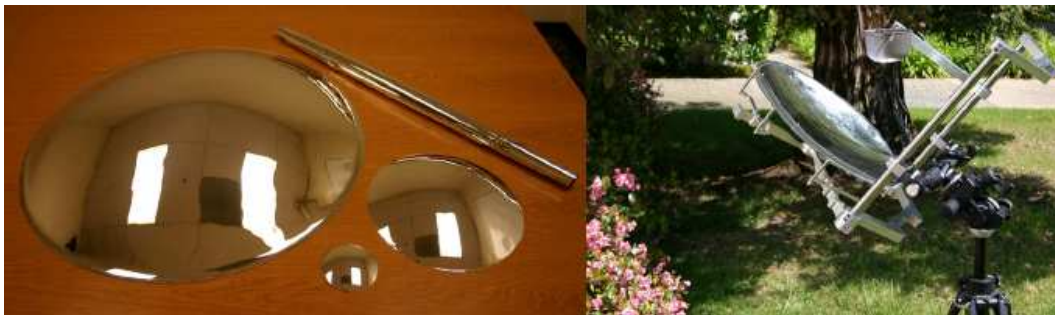
Figure 2.10: Mevicon form stiffened shell lightweight mirrors ©Mevicon Inc., used with permission.
