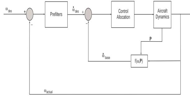
Figure 1: Block Diagram of Inner-loop Dynamic Inversion Control Law
