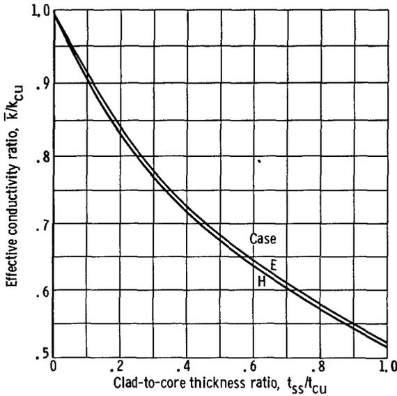
Figure 4 - Exact effective conductivity ratio against thickness ratio.
