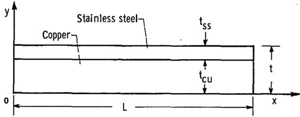
(b) As considered in analysis (thickness exaggerated).
