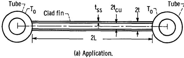
The configuration to be analyzed is shown in figure 1. This is a stainless-steel-clad copper fin such as might be used in a central fin-tube radiator (fig. 1(a)). Only one quarter of the fin is analyzed (fig. 1(b)) because symmetry is assumed about  $x = L$  and  $y = 0$ . There is no heat flow across these boundaries. The temperature at  $x = 0$  is assumed constant and equal to the tube outer-surface (base) temperature in a fin-tube configuration.
