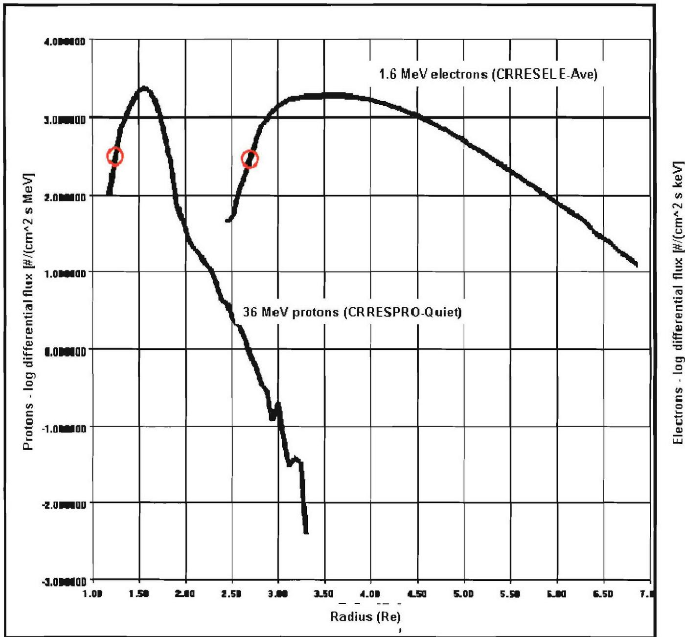
Figure 5. Radial Profiles Of the 36 Mev Protons and 1.6 Mev Electrons as Given by the CRRES PRO Quiet and CRRESELE Ave Models, Respectively. Red circles indicate the points used to estimate the maximum gradients.
