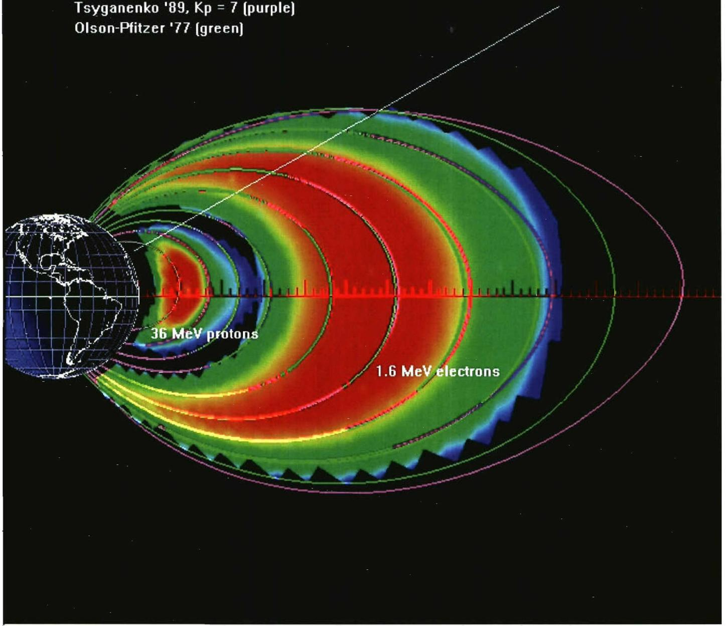
Figure 4. Cross Section of the Earth's Magnetosphere Showing Field Lines from the IGRF/Olson-Pfitzer '77 (green) and IGRF/Tsyganenko '89 (purple) Models. Field lines from both models intersect along the 0 deg longitude, 30 deg latitude radial line (white.)
