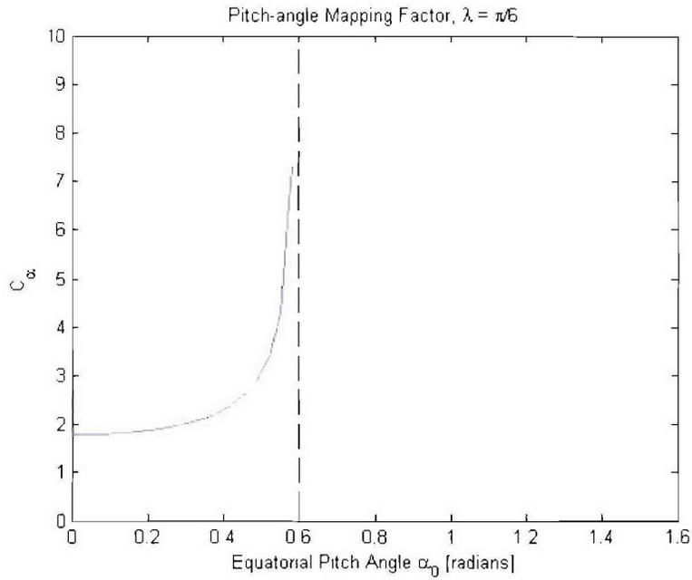
Figure 7. Pitch Angle Mapping Factor  $C_\alpha$  as a Function of Equatorial Pitch Angle for Magnetic Co-Latitude of  $\pi/6$  (30 degrees). The mirror angle is  $\sim 0.6$  radians ( $\sim 34$  degrees).
