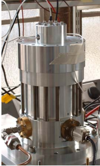
Figure 1 Test Rig Used For Gas Spring Loss Measurements
