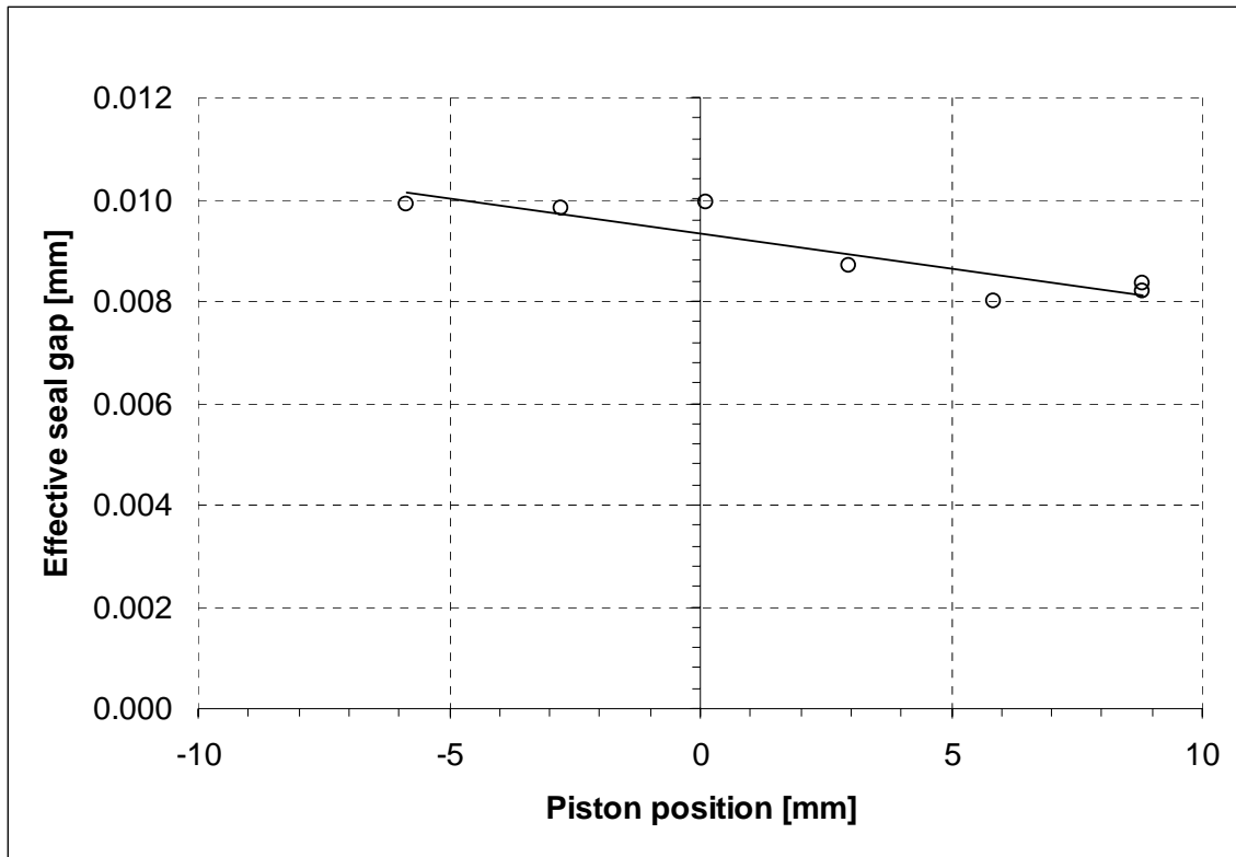
Figure 3 Variation of Seal Radial Clearance with Piston Position
