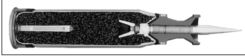
Figure 1. A cut away of large-caliber ammunition showing piccolo tube.
