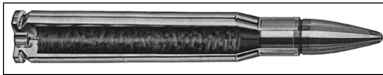
Figure 2. Cut away of a 5.56-mm small-caliber round.
