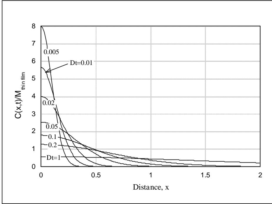
Figure 3. Concentration-distance curves for the thin-film solution.
