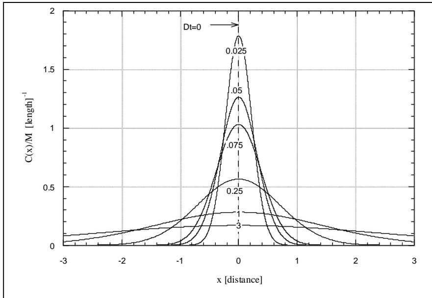
Figure 2. Concentration-distance curves for an instantaneous plane source.
