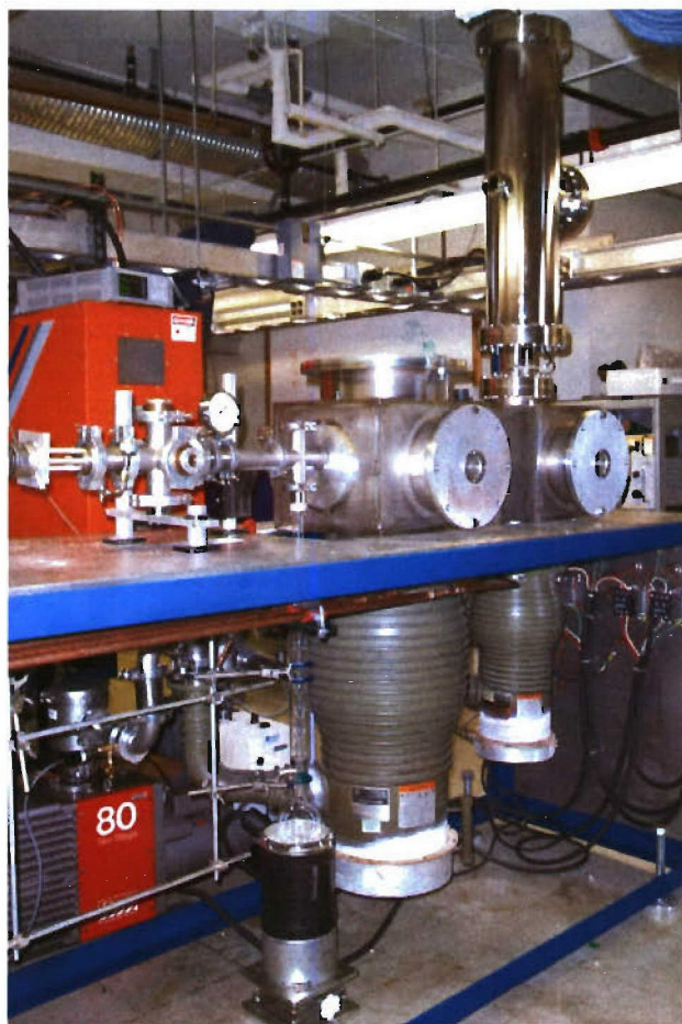
Figure 6. The laser vaporization flow-tube apparatus with on-line mass spectrometer system.
