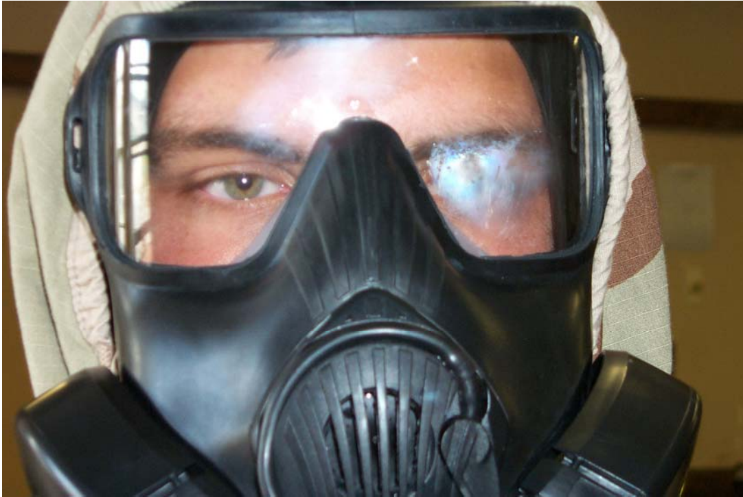
Figure 25. Soldier's XM50 mask fogging because of missing interior valve disk.
