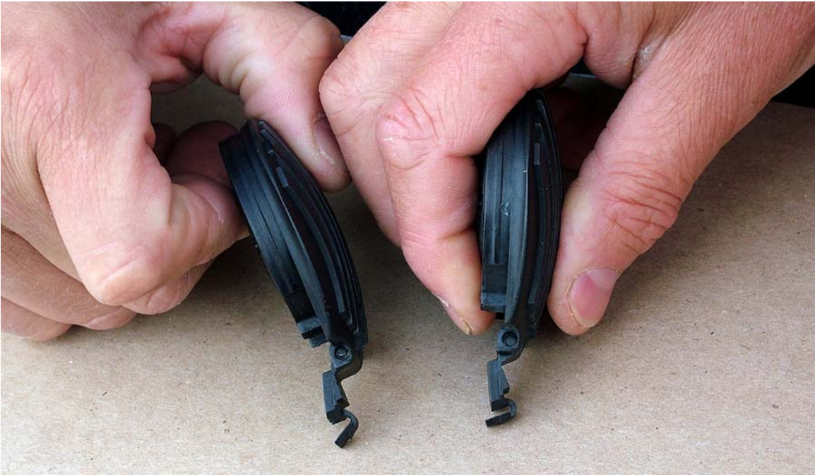
Figure 29. XM50 mask front module cover communication device flexed while the Soldier was attempting to remove the drink tube from the drink tube housing assembly.
