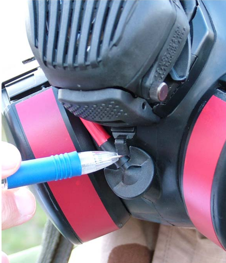
Figure 30. XM50 mask with modified mask beard voice amplifier push tab (bottom).
