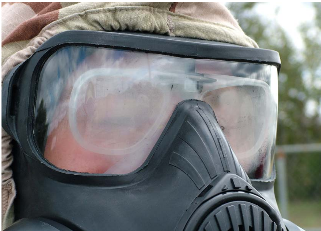
Figure 23. Soldier's XM50 mask fogging while he wore vision correction inserts (side view).
