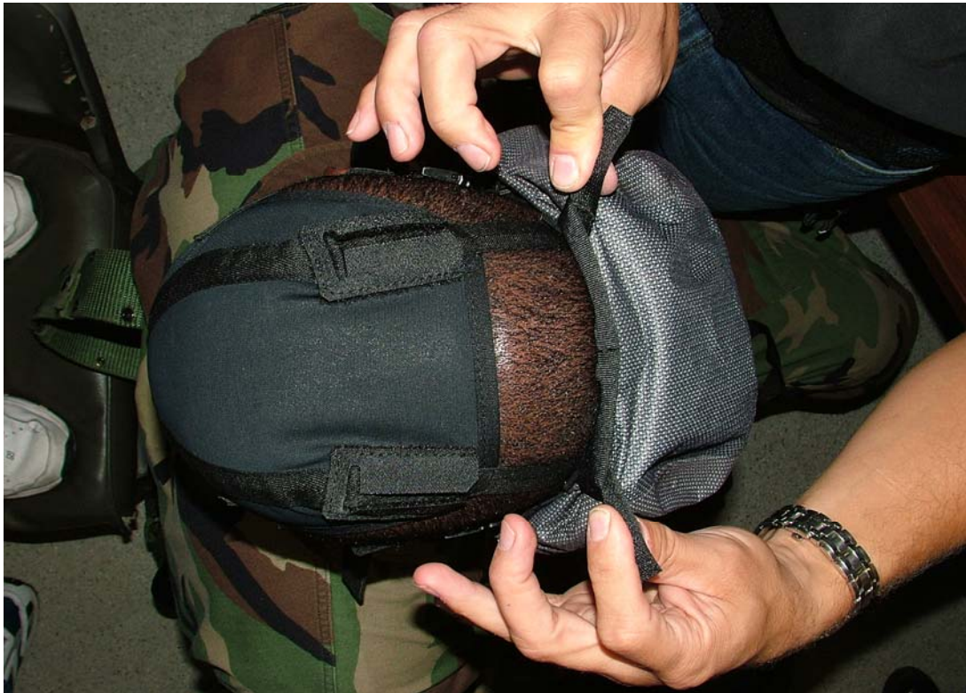
Figure 19. XM51 hood material bunching up after being fitted.
