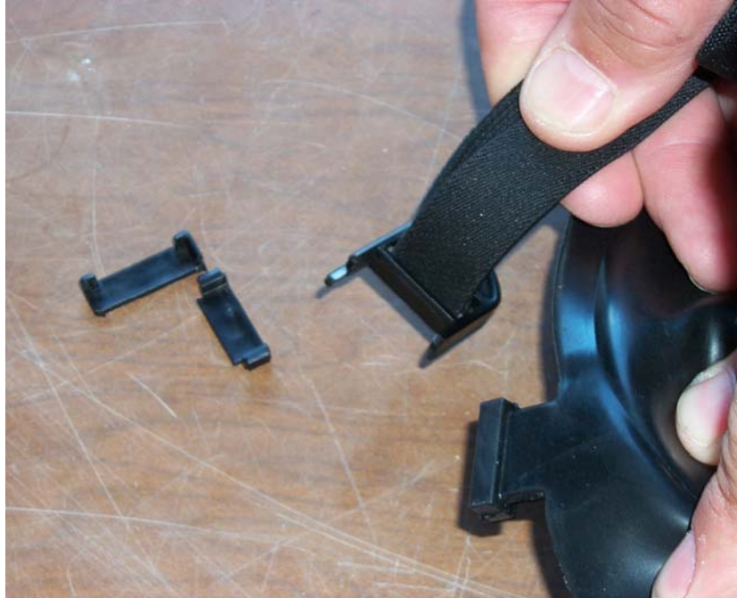
Figure 15. Broken XM50 mask temple strap clip buckle fastener.
