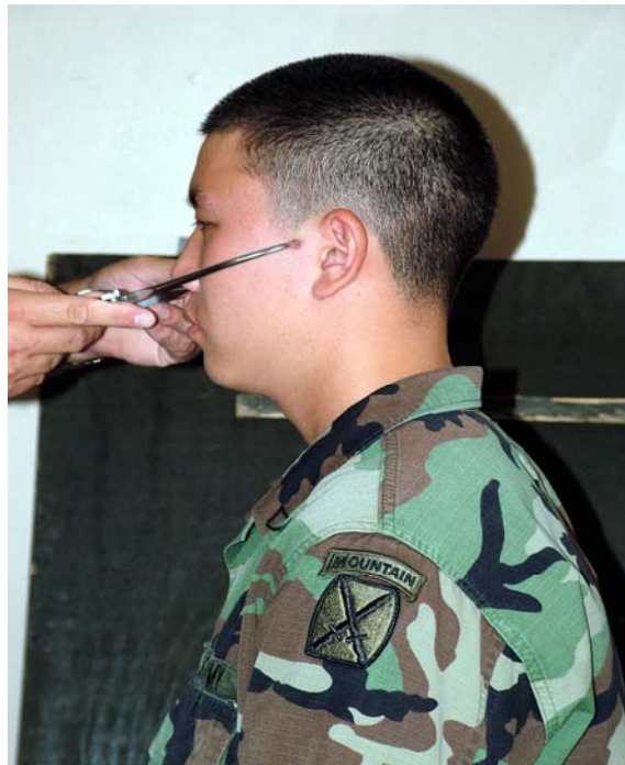
Figure 2. Anthropometry measurement of Soldier bizygomatic breadth.
