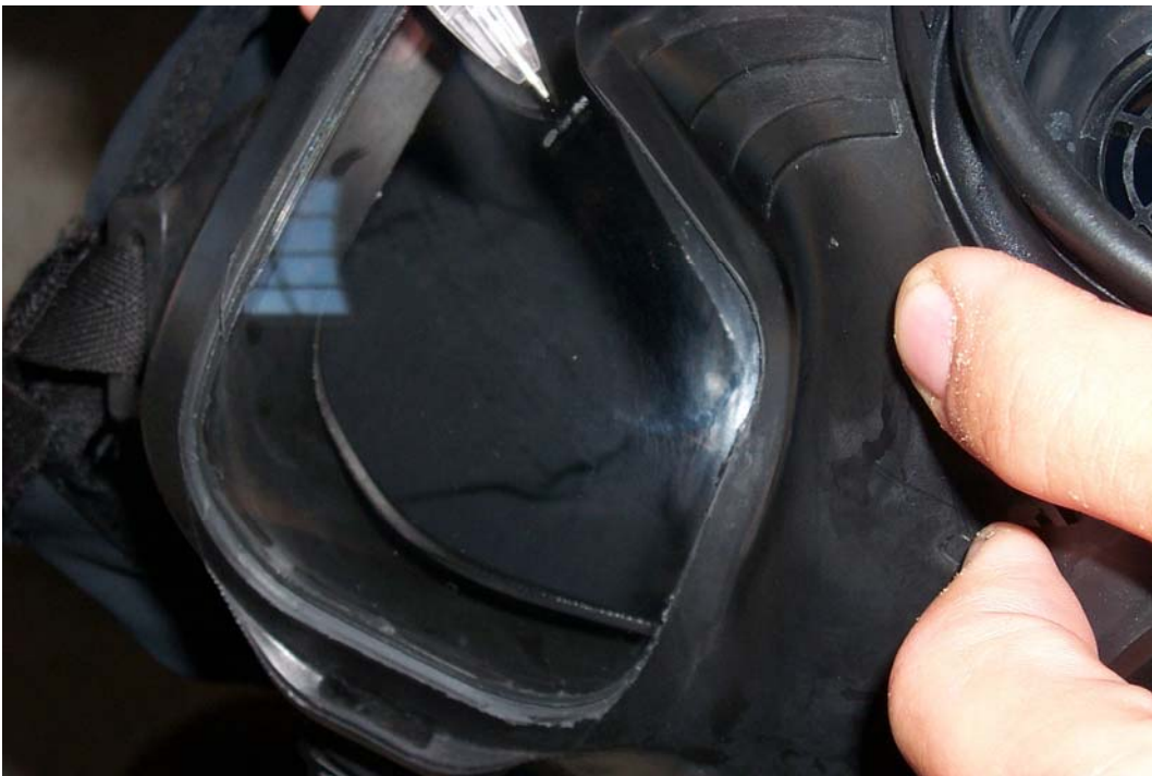
Figure 32. XM50 mask with two marks on the outer eye lens.
