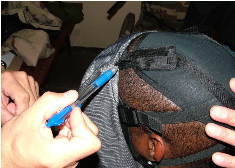
Figure 16. Brow straps adjusted beyond recommended setting.
