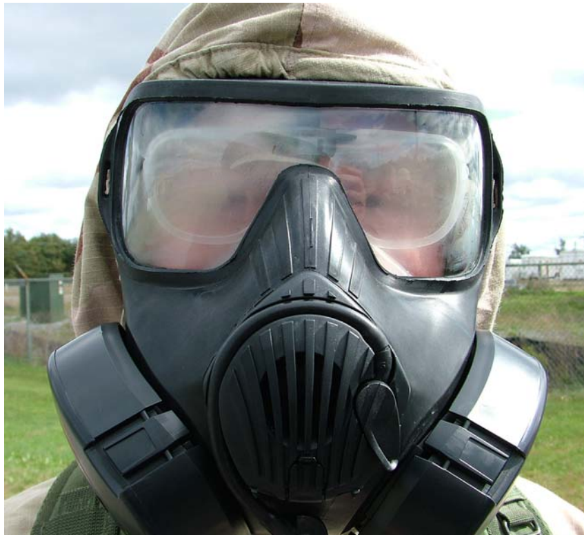
Figure 22. Soldier's XM50 mask fogging while he wore vision correction inserts.
