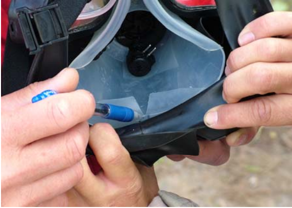
Figure 27. Inside view of XM50 nose-cup after fluid build-up.
