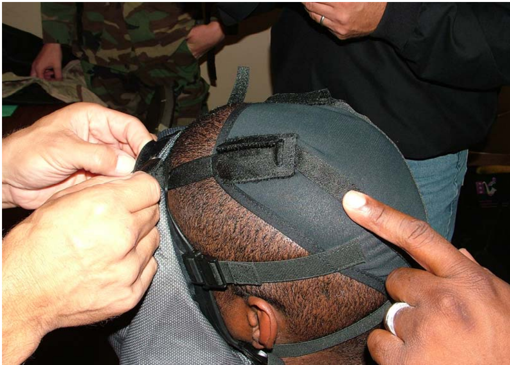
Figure 18. Brow straps adjusted beyond recommended setting (left side view).
