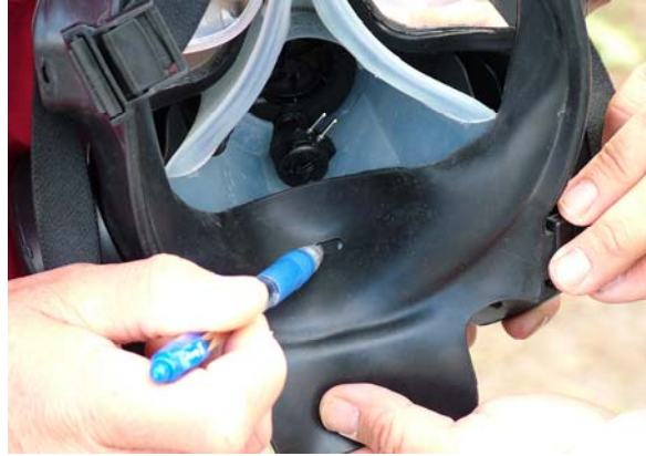
Figure 28. Inside view of XM50 mask chin cup pocket after fluid build-up.
