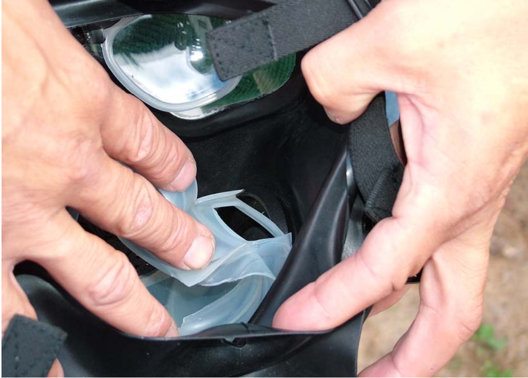
Figure 24. XM50 mask air flow management system not properly seated into the filter housing.
