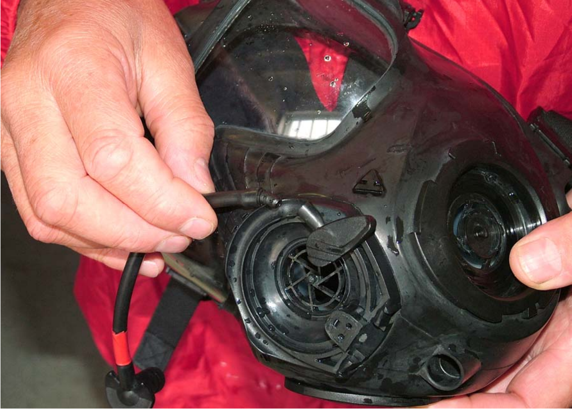
Figure 31. XM50 mask drink tube hose assembly detached from the drink tube housing assembly.
