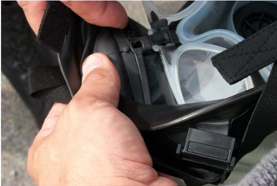
Figure 26. XM50 mask vision correction inserts were not connected to the holding pin.
