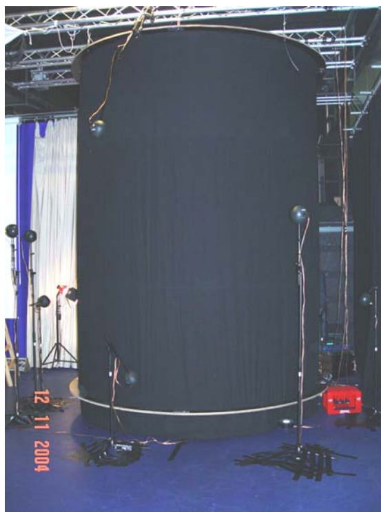
Figure 3.5: Picture of the curtain cylinder with loudspeakers mounted around it.
