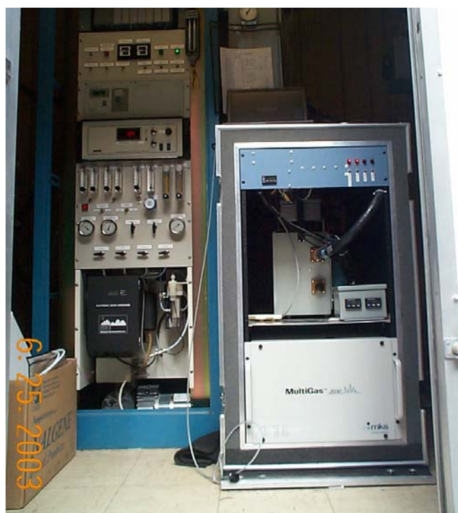
Figure 2: Mobile unit 1 in emission shed (right) and USCD's CLD instrument (left).
