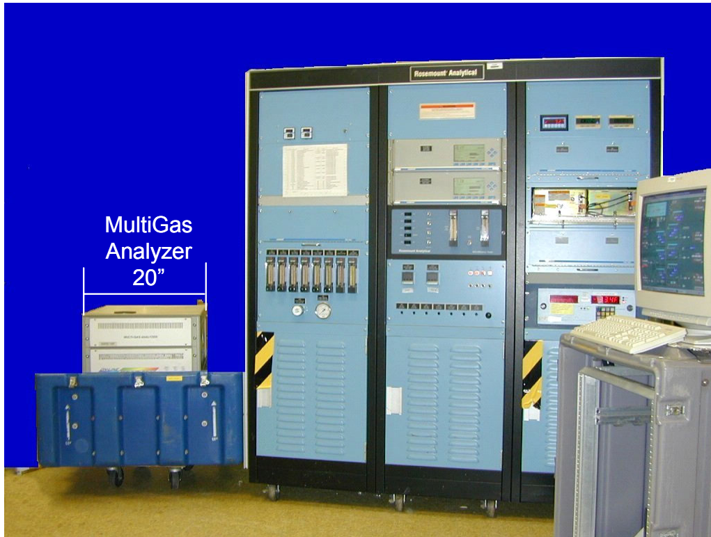
Figure 1: An FT-IR MultiGas Analyzer (MGA), in a convenient shipping case, next to a traditional gas analysis system. The much smaller MGA measures more gases for a fraction of the traditional capital and maintenance costs [1-3] Photograph courtesy of Vince Zaccardi, Jacobs-Sverdrup/AEDC Group.
